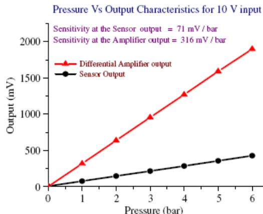
**Fig. 1 Summary of Results on the packaged pressure sensors [16]**
