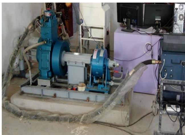
**Fig.2 Four-stroke single cylinder computerized diesel engine test rig**
