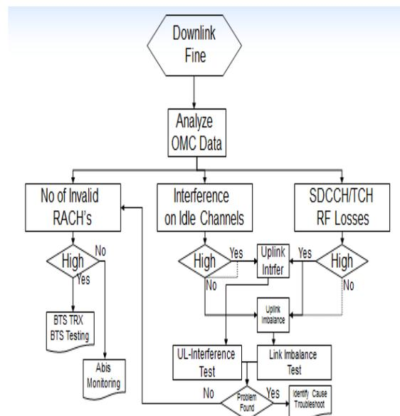
**Fig.5 Block Diagram Showing RACH Non Detection**
