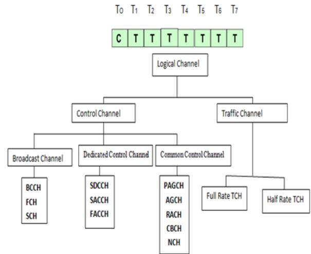
**Fig. 1. Diagram Showing Logical Channels Classification**
