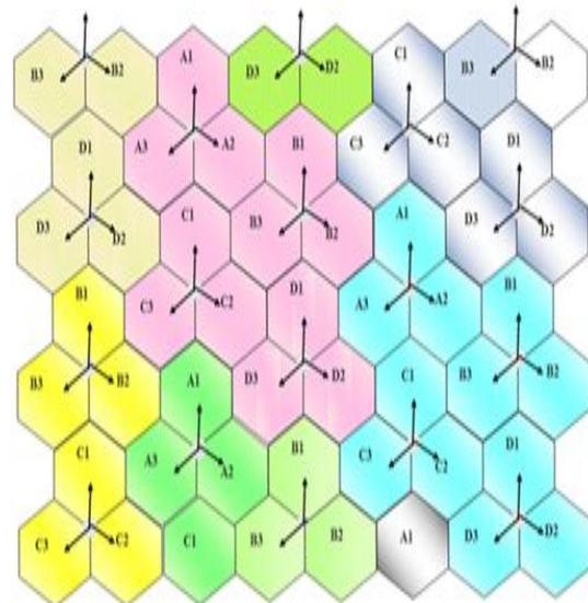
**Fig. 4. Diagram Showing 4/12 Reuse Patterns**
