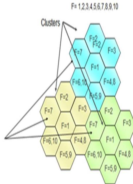
**Fig.2 Diagram Showing Frequency Re-use Pattern Objective:**
