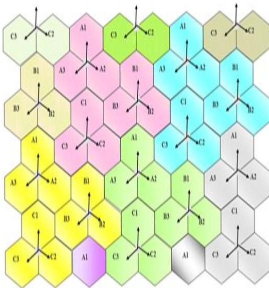
**Fig. 3. Diagram Showing 3/9 Frequency Re-use Pattern**
