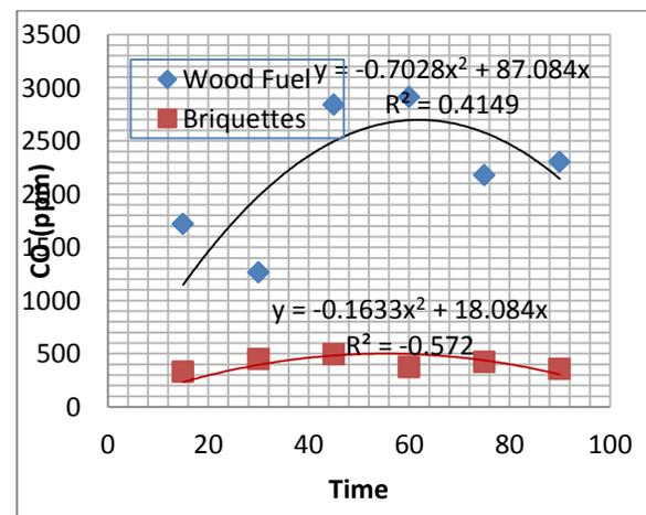
Figure 5: Carbon Monoxide Emission Profiles for briquettes and wood fuel
