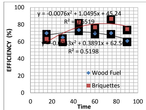
Figure 4: Comparing boiler combustion efficiency of briquette and wood fuel
