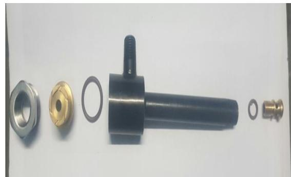
**Fig 3: Fabricaed components of vortex tube**
