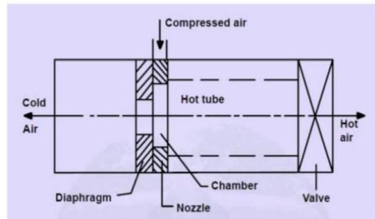
**Fig 1: Schematic showing major components of vortex tube**
