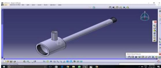
**Fig 4: Main body of vortex tube**
