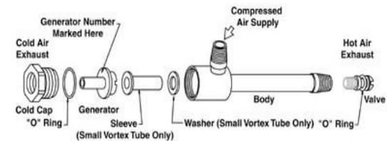
**Fig 2: Disassembled components of vortex tube**
