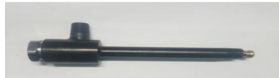
**Fig 8: Fabricated Vortex tube**
