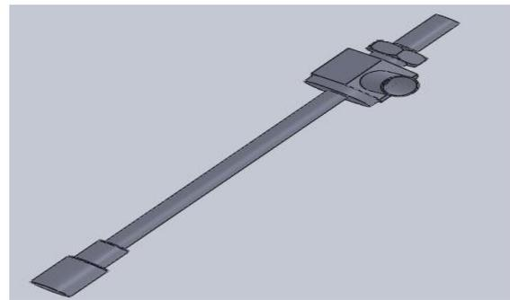
**Fig 7: Isometric view of vortex tube**
