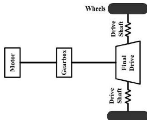
**Fig 1. Integrated Motor Transmission Powertrain**
