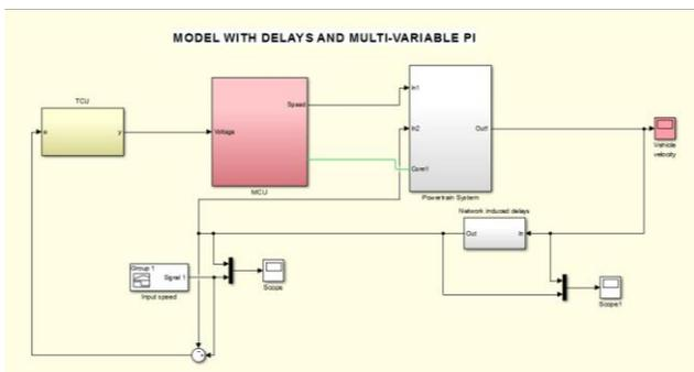
**Fig 3. Simulation diagram for IMT powertrain system**
