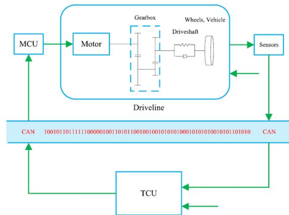
**Fig 2. Control architecture via CAN**
