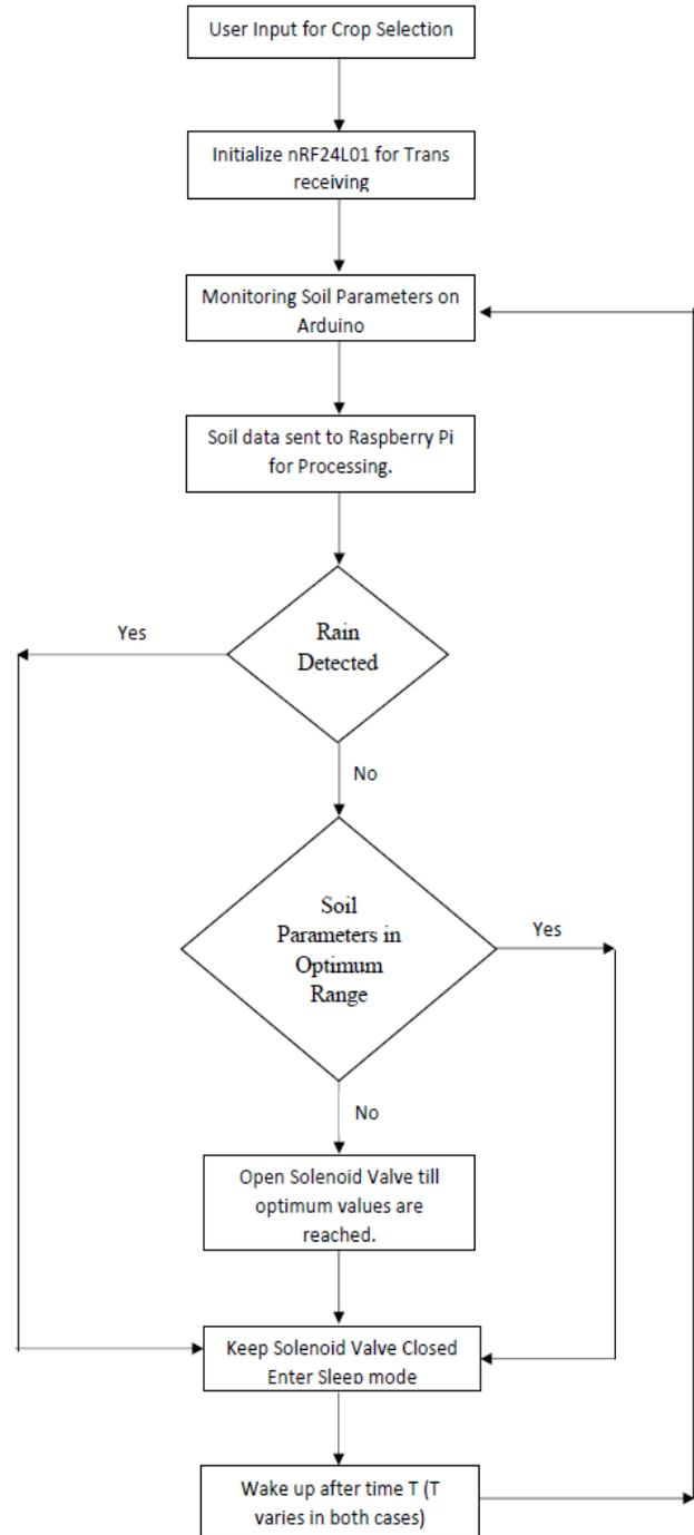
**Figure 2. Design Algorithm**
