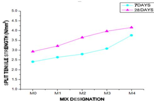
**Fig 6: Performance of fibers on split tensile strength**
