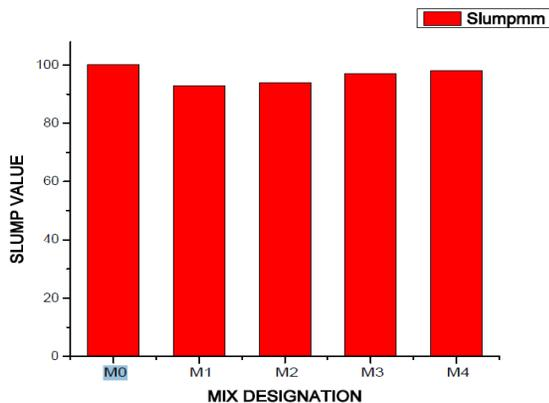
**Fig 3: Variation of slump for different mixes**
