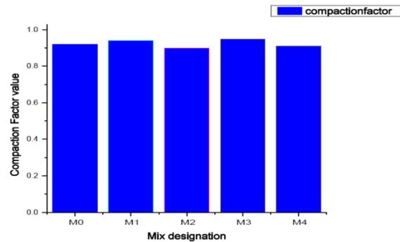
**Fig4: Variation of compaction factor for different mixes**
