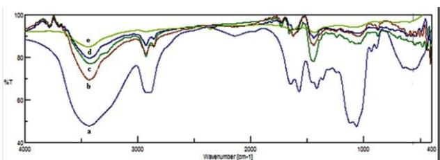
**Fig (1): FTIR for a) CMC , b) CMC:PVA (1:1) , c) CMC:PVA (2:1), d) CMC:PVA (1:2) and e) PVA.**
