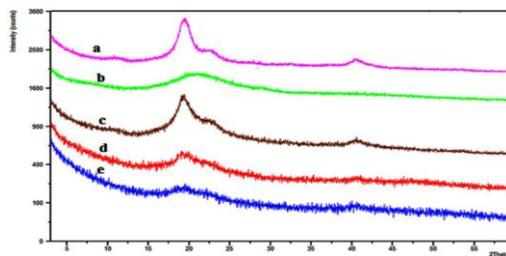
**Fig (2): X-Ray Diffraction for a) PVA, b) CMC, c) CMC: PVA (1:2), d) CMC: PVA (2:1) and e) CMC:PVA (1:1).**
