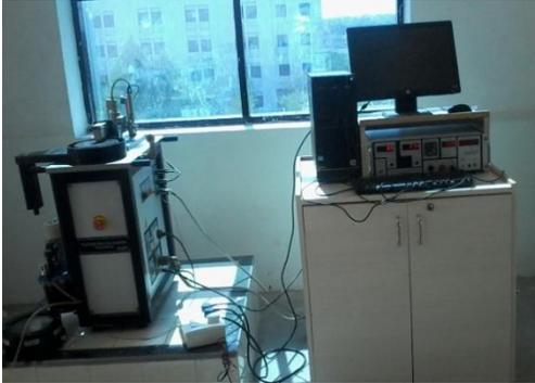
**Figure 5.1 Friction Wear Monitor with Computer & Display Panel**
