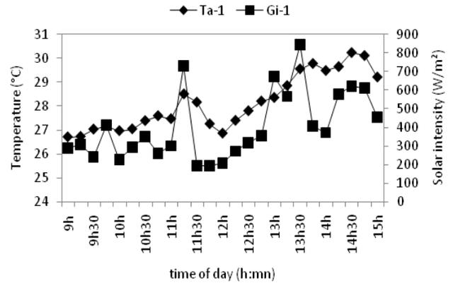
**Fig. 2** Environmental condition as of 24/06/2016: (♦ Ta-1) ambient temperature, (■ Gi-1) global instantaneous radiation
