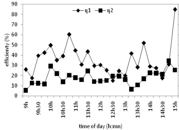
**Fig. 7 Profiles of collector efficiency in condition 1 ( $\eta_1$ ) and in condition 2 ( $\eta_2$ )**
