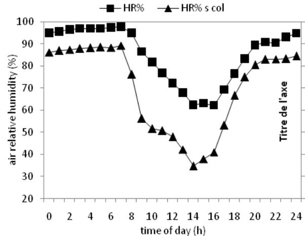
**Fig. 10 Profiles of the mass of water vapour in 1 kg of dry air for ambient and outlet the collector**
