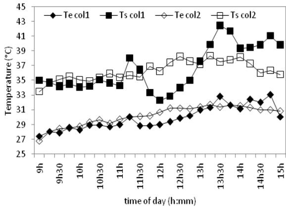
**Fig. 6 Profiles of temperature in inlet and outlet of collector**
