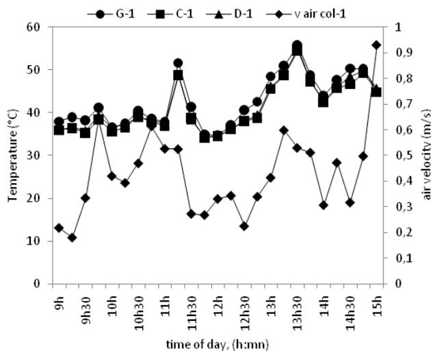
**Fig. 4 Profiles in upper channel: temperature in the collector width at 30 cm from the inlet and average air flow velocity at this inlet during condition 1 (24/06/2016)**
