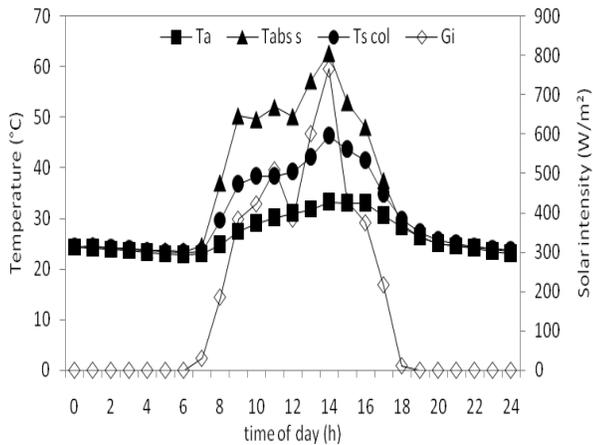
**Fig. 8 Profiles of temperatures out and in the collector and global instantaneous radiation**
