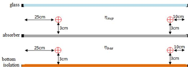
**Fig. 1** Position of the thermo-hygrometric and air velocity probes in the collector (inlet and outlet) in the longitudinal direction
