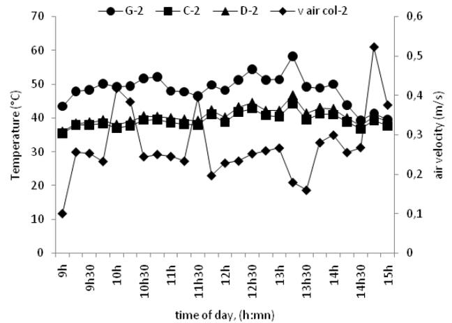
**Fig. 5 Profiles in upper channel: temperature in the collector width at 30 cm from the inlet and average air flow velocity at this inlet during condition 2 (27/06/2016)**
