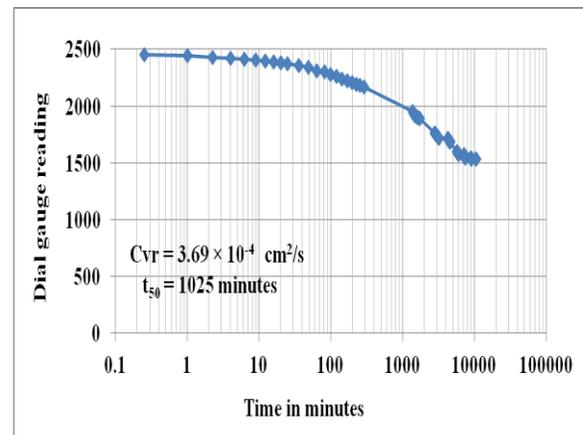
Figure 7 Settlement versus log t characteristics of soft Kaolinite clay during consolidation through radial drainage (Hydraulic pressure 320 kPa)
