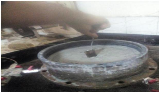
**Figure-3 Photograph Showing Installation of Band Drain**
