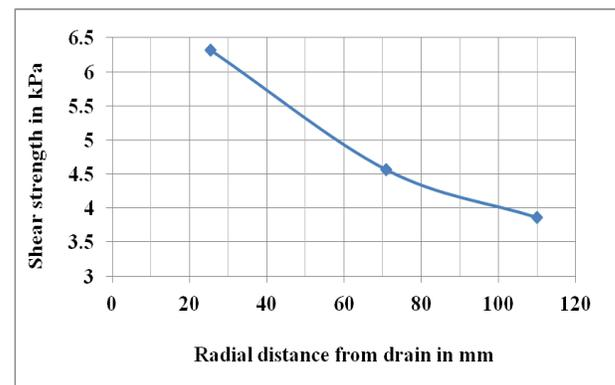
**Figure 15 Radial distance versus shear strength curve for Kaolinite clay during consolidation by radial drainage using Vacuum (10 minutes interval)**
