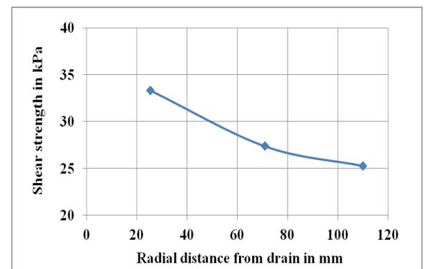
Figure 11 Radial distance versus shear strength curve for Kaolinite clay during consolidation by radial drainage
