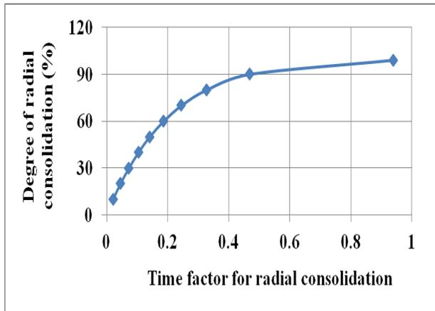
Figure 5 Degree of consolidation versus time factor characteristics for consolidation of Kaolinite clay through radial drainage
