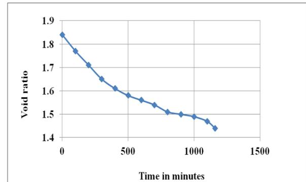
**Figure 18 Void ratio versus time curve characteristic during consolidation of Kaolinite clay through radial drainage using Vacuum (20 minutes interval)**
