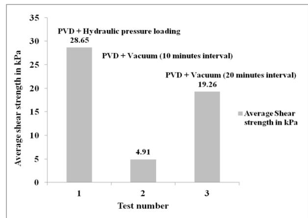
**Figure 22 Comparison of Average shear strength during consolidation of Kaolinite clay through radial drainage using Hydraulic pressure loading and Vacuum**
