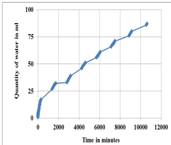
Figure 9 Quantity of water squeezed versus time characteristic during consolidation of Kaolinite clay through radial drainage (Hydraulic pressure 320 kPa)
