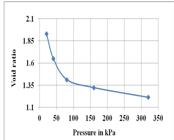
Figure 10 Void ratio versus pressure curve for Kaolinite clay during consolidation by radial drainage
