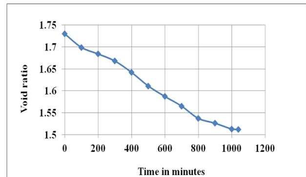
**Figure 14 Void ratio versus time curve characteristic during consolidation of Kaolinite clay through radial drainage using Vacuum (10 minutes interval)**
