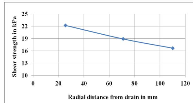
**Figure 19 Radial distance versus shear strength curve for Kaolinite clay during consolidation by radial drainage using Vacuum (20 minutes interval)**
