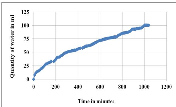
**Figure 13 Quantity of water expelled versus time characteristic during consolidation of Kaolinite clay through radial drainage using Vacuum (10 minutes interval)**
