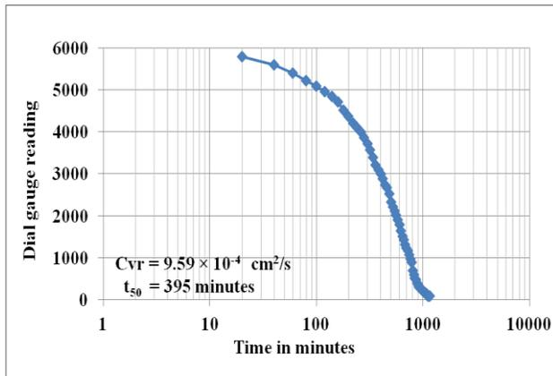
**Figure 16 Settlement versus log t characteristics of soft Kaolinite clay during consolidation through radial drainage (Vacuum 85.68 kPa)**
