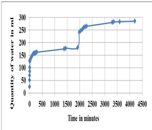
Figure 8 Quantity of water squeezed versus time characteristic during consolidation of Kaolinite clay through radial drainage (Hydraulic pressure 20 kPa)
