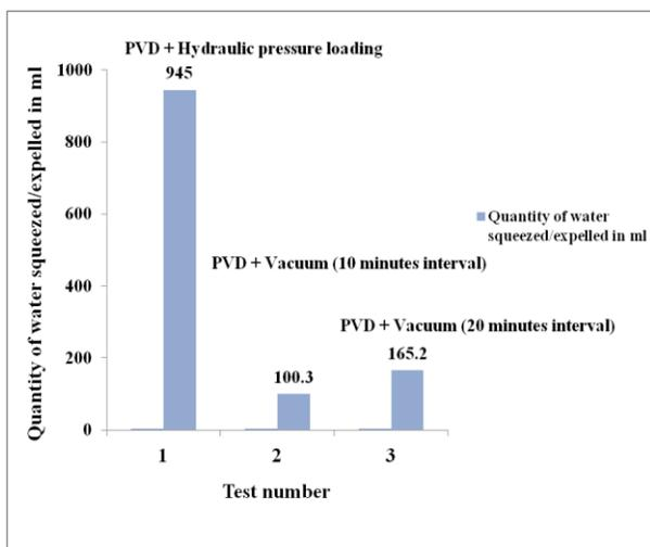
**Figure 21 Comparison of Quantity of water squeezed/expelled during consolidation of Kaolinite clay through radial drainage using Hydraulic pressure loading and Vacuum**
