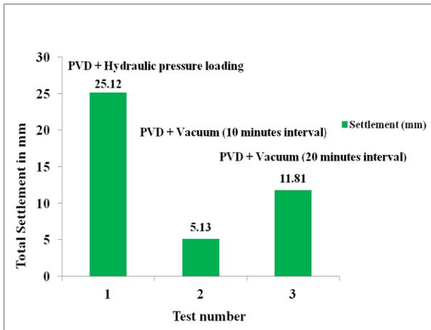
**Figure 20 Comparison of total settlement during consolidation of Kaolinite clay through radial drainage using Hydraulic pressure loading and Vacuum**
