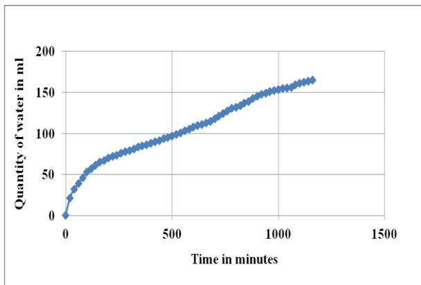
**Figure 17 Quantity of water expelled versus time characteristic during consolidation of Kaolinite clay through radial drainage using Vacuum (20 minutes interval)**
