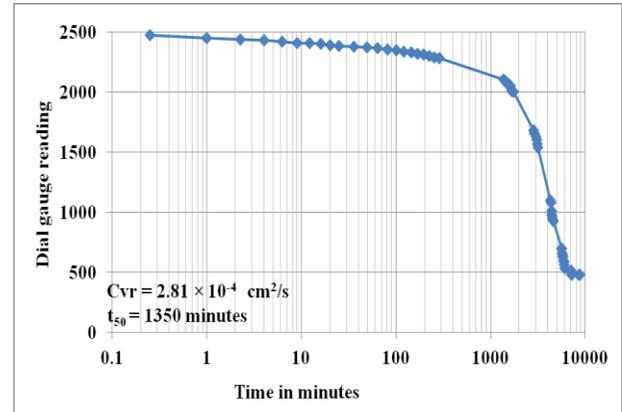
Figure 6 Settlement versus log t characteristics of soft Kaolinite clay during consolidation through radial drainage (Hydraulic pressure 20 kPa)
