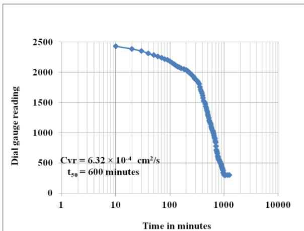
**Figure 12 Settlement versus log t characteristics of soft Kaolinite clay during consolidation through radial drainage using Vacuum (Vacuum 85.68 kPa, 10 minutes interval)**
