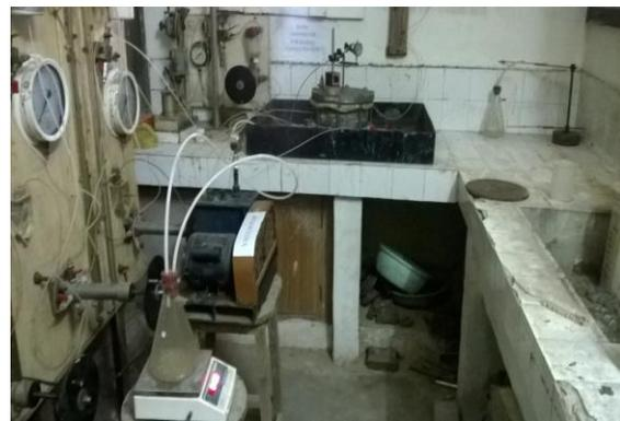
**Figure-2 Arrangement Showing Vacuum Pump Connection with Rowe Type Oedometer through Conical Flask**
