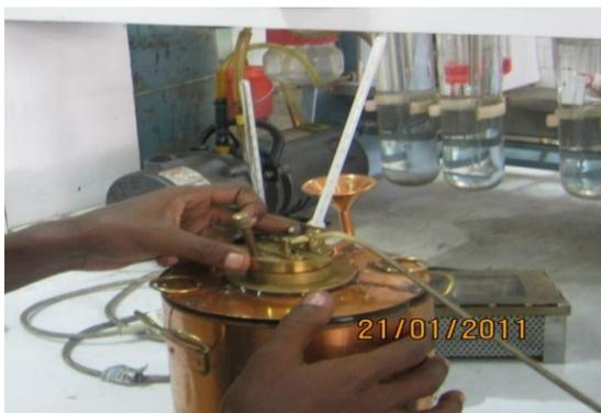
**Figure 9: Closed-cup IP-170 flash-point measuring device**
