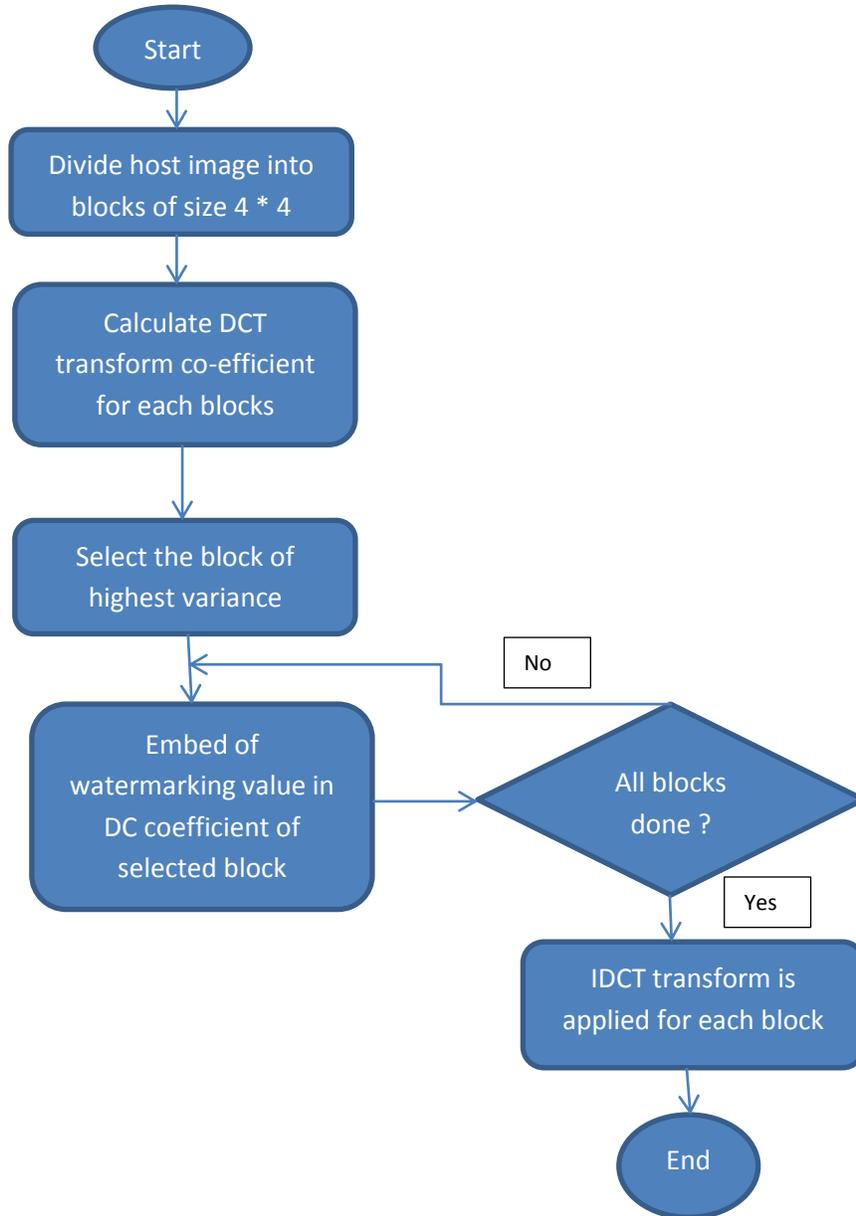
**Figure 2: The DCT algorithm flow chart**
