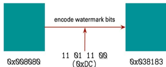
**Figure 4 Encoding of watermark bits**
