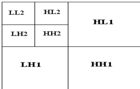
**Figure3 Two-level DWT**
