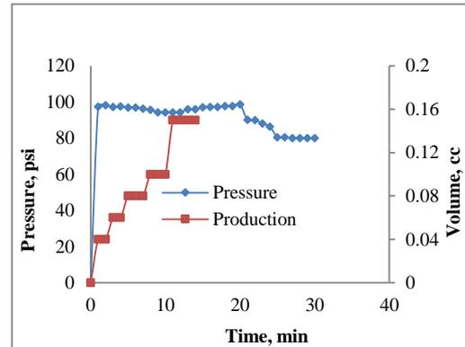
**FIGURE IX CORE #2 SURFACTANT FLOODING PRESSURE AND PRODUCTION PROFILES**
