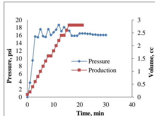
**FIGURE III CORE #3 WATERFLOODING PRESSURE AND PRODUCTION PROFILES**
