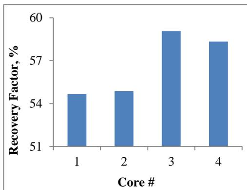
**FIGURE V COREPLUGS WATERFLOODING RECOVERY FACTORS**
