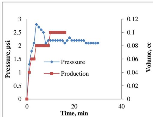
**FIGURE VIII CORE #1 SURFACTANT FLOODING PRESSURE AND PRODUCTION PROFILES**
