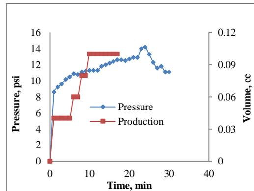
**FIGURE X CORE #3 SURFACTANT FLOODING PRESSURE AND PRODUCTION PROFILES**
