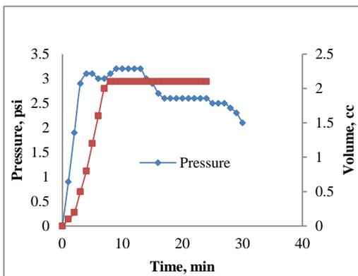
**FIGURE 1 CORE #1 WATERFLOODING PRESSURE AND PRODUCTION PROFILES**
