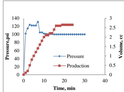
**FIGURE 2 CORE #2 WATERFLOODING PRESSURE AND PRODUCTION PROFILES**
