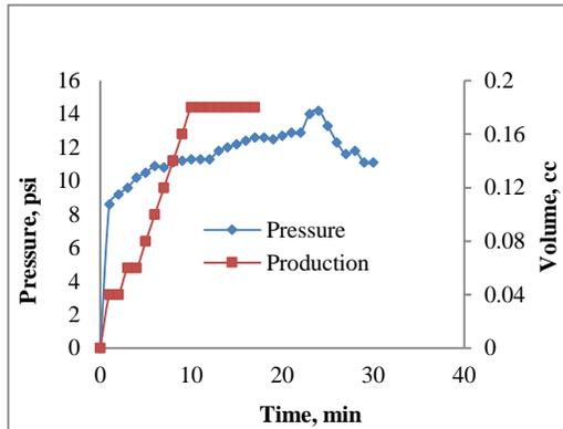
**FIGURE XI CORE #4 SURFACTANT FLOODING PRESSURE AND PRODUCTION PROFILES**
