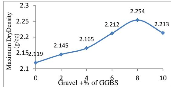
**Fig.6 Variation of MDD with Addition of Percentage GGBS to Gravel**
