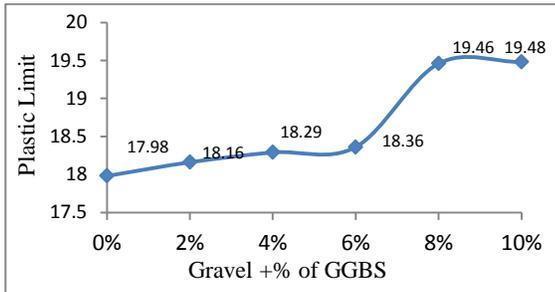
**Fig. 4. Variation of Plastic Limit with Addition of Percentage GGBS to Gravel**
