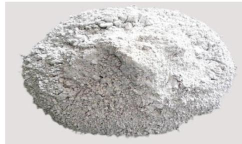
Fig. 2. Ground Granulated Blast Furnace Slag (GGBS)
