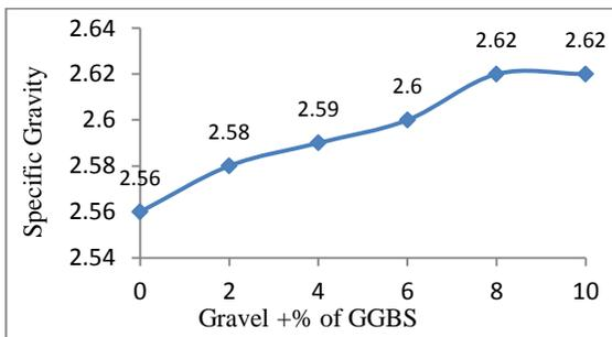
**Fig.5 Variation of Specific Gravity with Different Percentage GGBS Mixed in Gravel**
