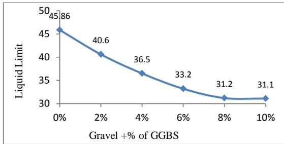
**Fig.3. Variation of Liquid Limit with Addition of Percentage GGBS to the Gravel**
