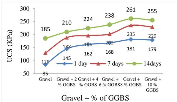
**Fig.9. Variation of Unconfined Compressive Strength with Different % of GGBS blending in Gravel at Different Curing Periods**
