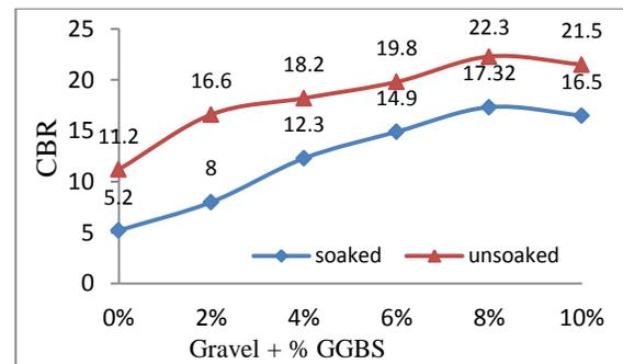
**Fig.8 Effect of Different % of GGBS on Unsoaked and Soaked CBR Mixed in Gravel**
