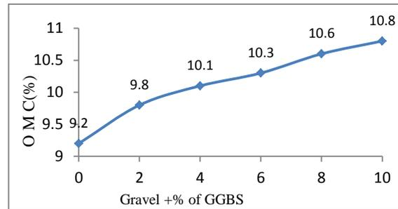
**Fig.7 Variation of OMC with addition of percentage GGBS to Gravel**
