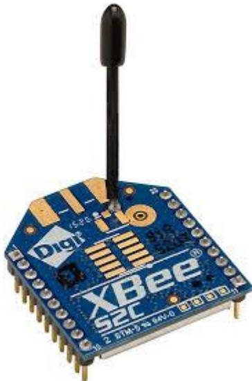
Figure: Zigbee Module
