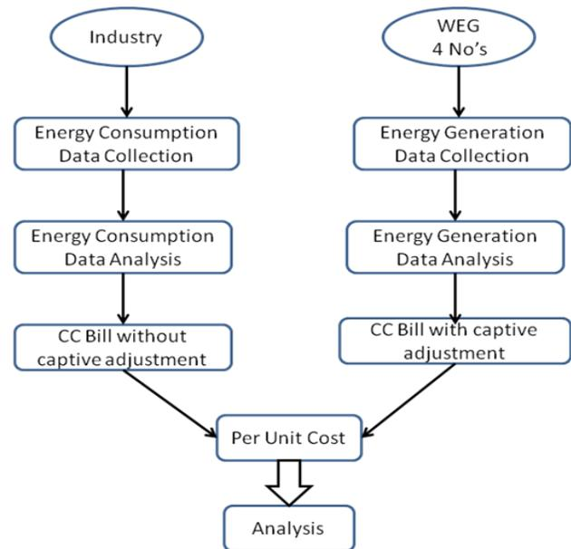
**Figure.1 Proposed flow model of audit work**
