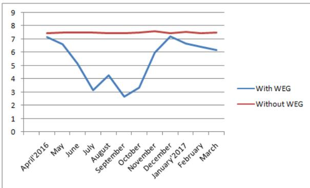
**Figure.4 Per unit cost comparison with and without WEG units**
