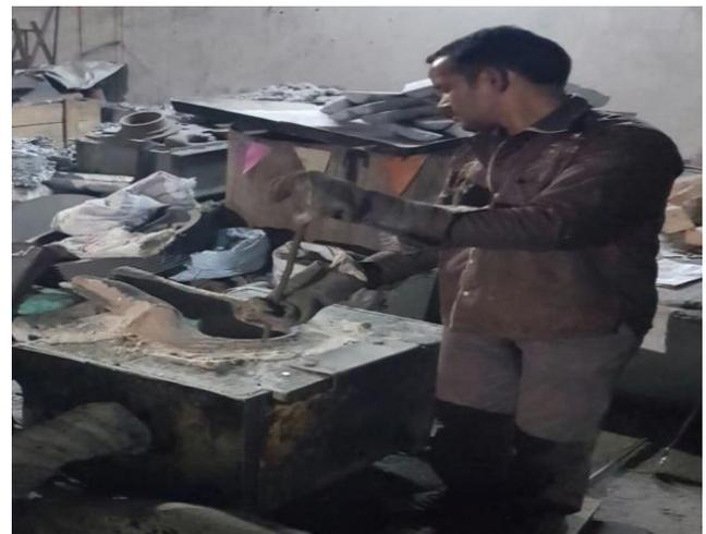
**Figure 2: Performing Manual Stir Casting**
