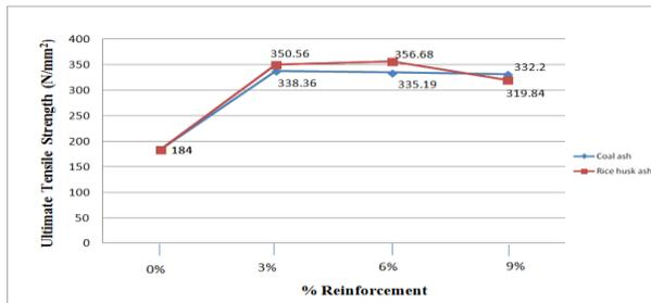
**Graph 04: Comparison of Ultimate Tensile Strength and % Reinforcement**
