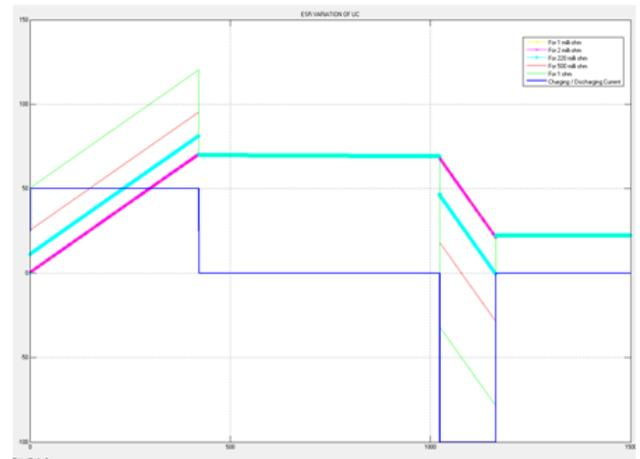
**Figure 7: Ultracapacitor for Different Values of ESR (Voltage & Current Vs Time)**
