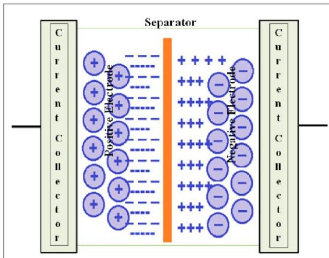
Figure 2: Schematic diagram of Ultracapacitor
