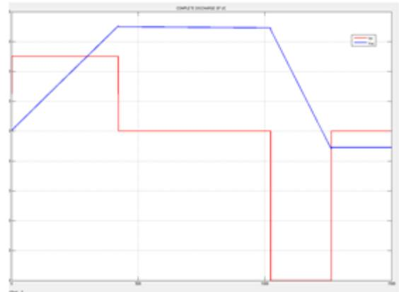
**Figure 6: Ultracapacitor with complete discharge (Voltage & Current Vs Time)**
