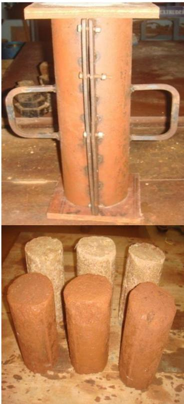
**Figure 2. Mould assembly compressed under UTM and samples obtained for UCS Testing**
