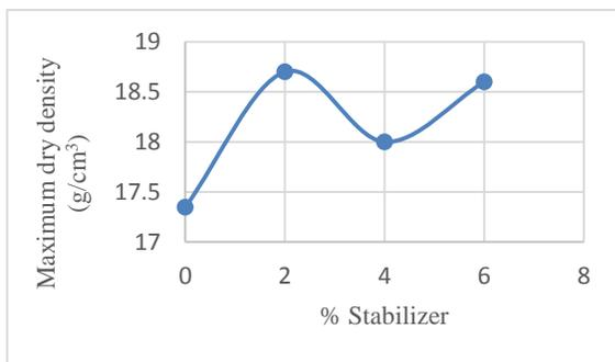
**Figure 5. Variation of Maximum Dry Density with different percentages of stabilizer for Shedi soil**
