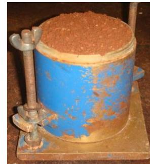
**Figure 1. Preparation of sample by IS Heavy Compaction to determine Maximum dry density and Optimum moisture content**
