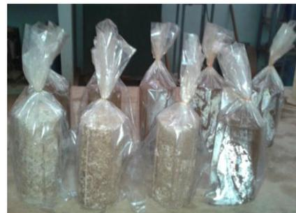
**Figure 3. Curing of samples prepared for Unconfined Compression Test**
