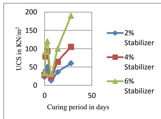
**Figure 8. Variation of UCS (soaked) with curing period for different percentages of stabilizer for Shedi soil**
