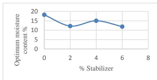
**Figure 6. Variation of Optimum Moisture Content with different percentages of stabilizer for Shedi soil**
