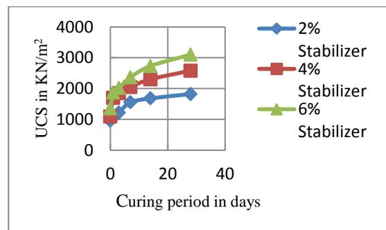
**Figure 7. Variation of UCS (unsoaked) with curing period for different percentages of stabilizer for Shedi soil**
