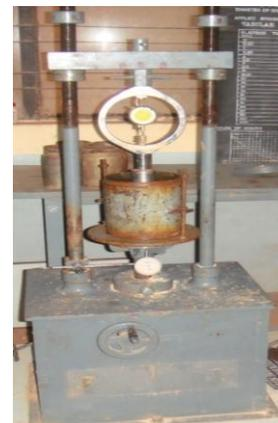
**Figure 4. California bearing ratio testing machine and the specimen undergoing testing.**
