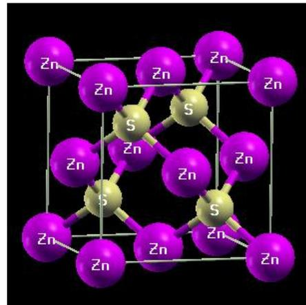
Fig.1 ZnS structure (as seen in XCrySDEN)
