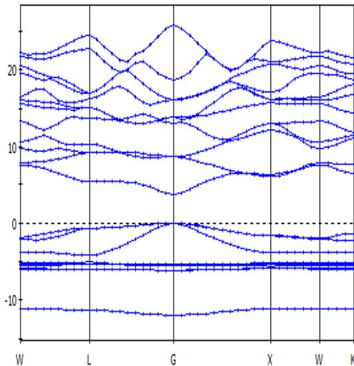
**Fig.2 Band Structure of ZnS**
