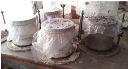
Fig. 2: 7days Curing of Unsoaked CBR Samples
