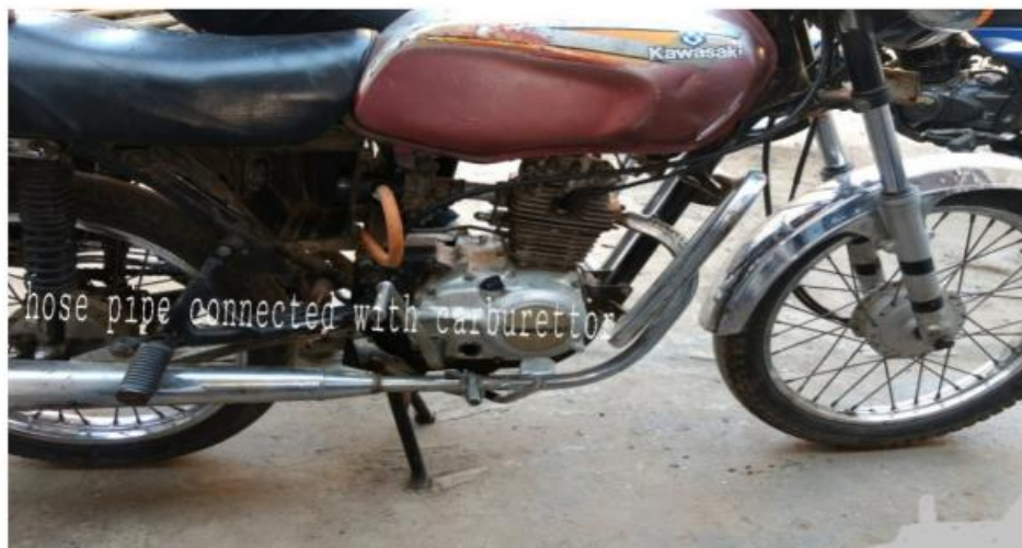
Fig -2 Fig shows how hose pipe connected with carburetor.
