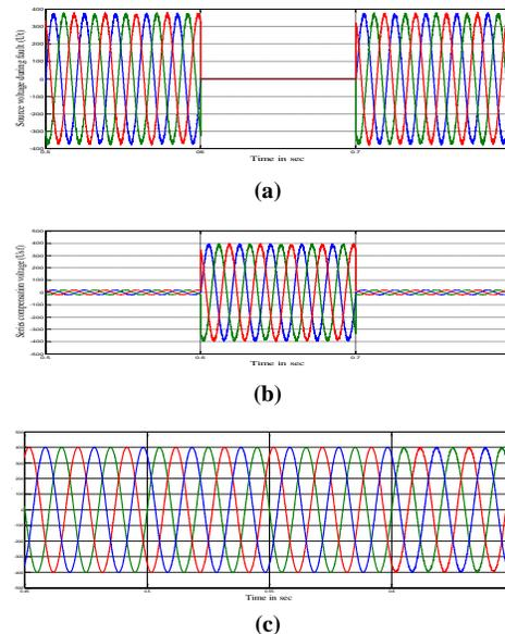
**Fig. 9 System performance during three phase to ground fault (a) supply voltage (b) UPQC injected voltage (c) Compensated load voltage**
