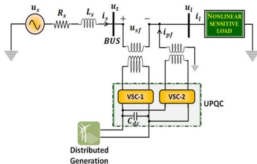
**Fig. 2 Simulated test system with multilevel converter**
