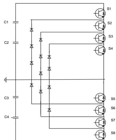
**Fig. 3 5level diode clamped multilevel converter**
