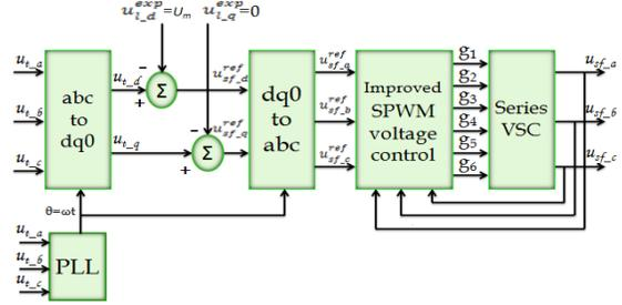
Fig. 7 Control block diagram of the series VSC
