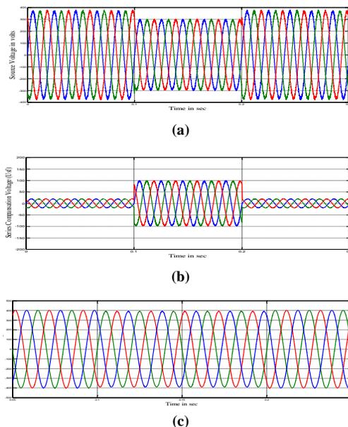
**Fig. 8 system compensation during sag (a) sag in supply voltage (b) UPQC injected voltage (c) Compensated load voltage**
