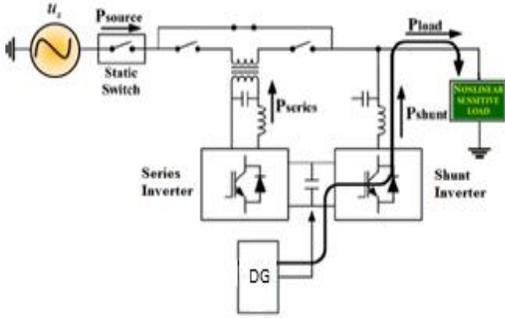
Fig. 6 UPQC-DG System operation with islanding mode
