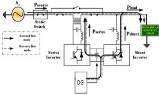
Fig. 5 UPQC-DG System operation with interconnected mode
