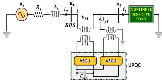
**Fig. 1 Basic configuration of the UPQC**
