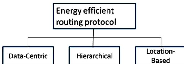
Figure 2: Classification of routing in WSNs
