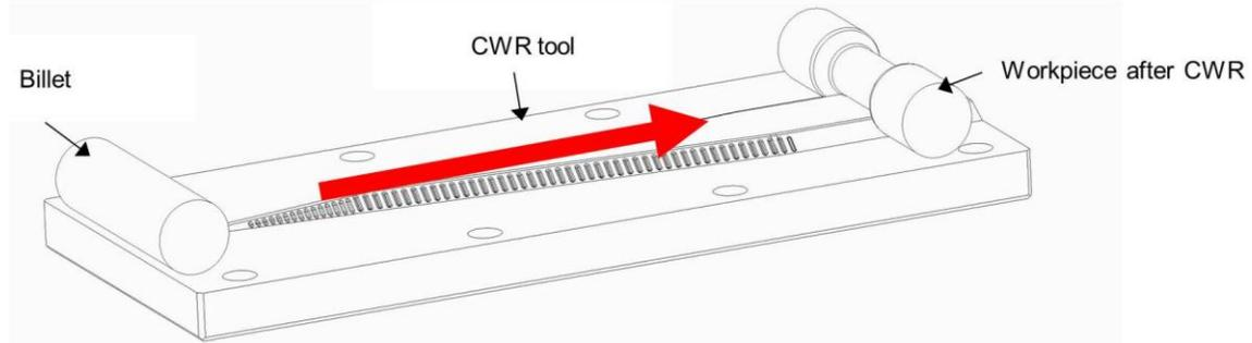
**Fig. 2: Scheme of the CWR process**
