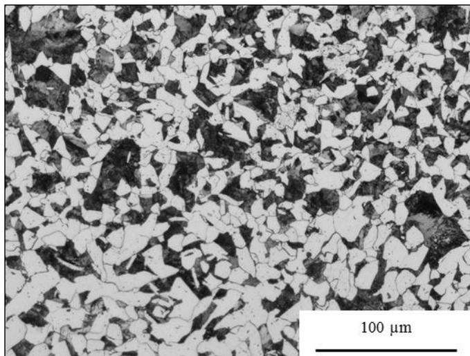
Figure 6: Microstructure of the coating after CWR, pointed in figure 4 as X
