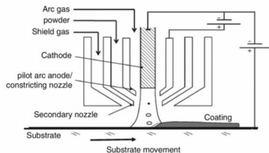
**Fig. 1: Scheme of the PTA process [3]**
