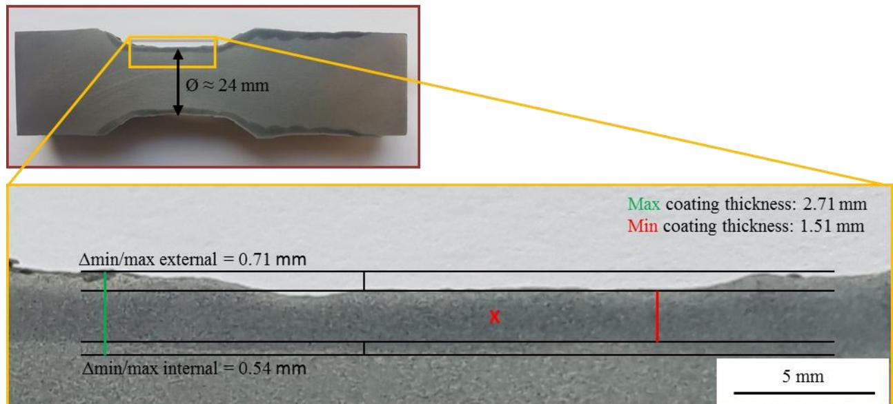
**Figure 4: Coating geometry after CWR**
