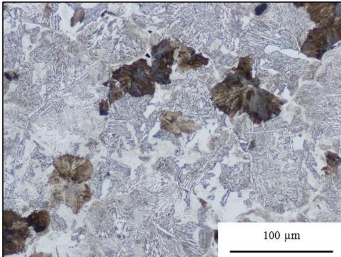
Figure 5: Microstructure of the coating as welded, pointed in figure 3 as X
