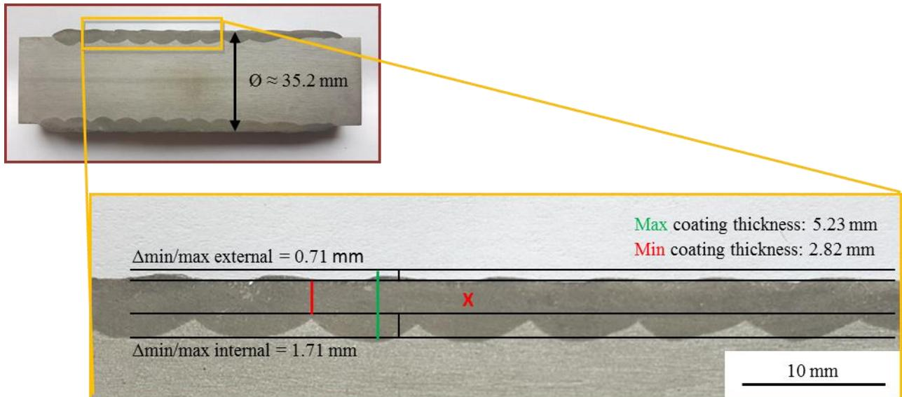
**Figure 3: Coating geometry after deposition welding**
