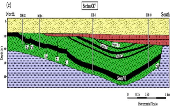
**Fig. 5: Cross section CC' of the Barapukuria Basin [7]**
