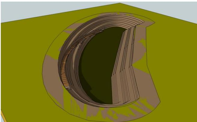
**Fig.11: 3-D view of the Ramp of the northern part of the Barapukuria Coal Field (SE View)**
