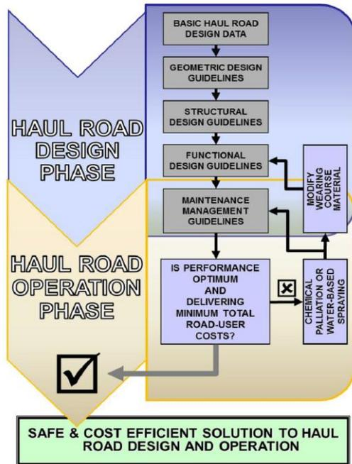
**Figure-2: Typical Haul Road Design & Operation Phases [After Thompson, Roger. 2011. Mine haul road design and management: a review of current practice.]**
