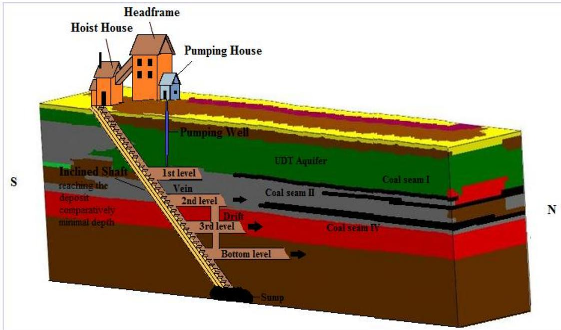
Fig 8: Underground mine system (Longwall)
