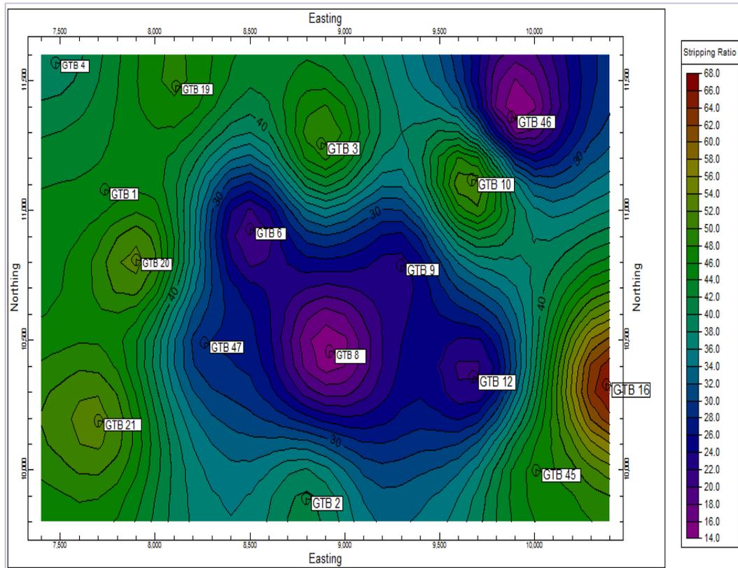
**Fig 7: Stripping ratio variation of coal seam I around the basin**
