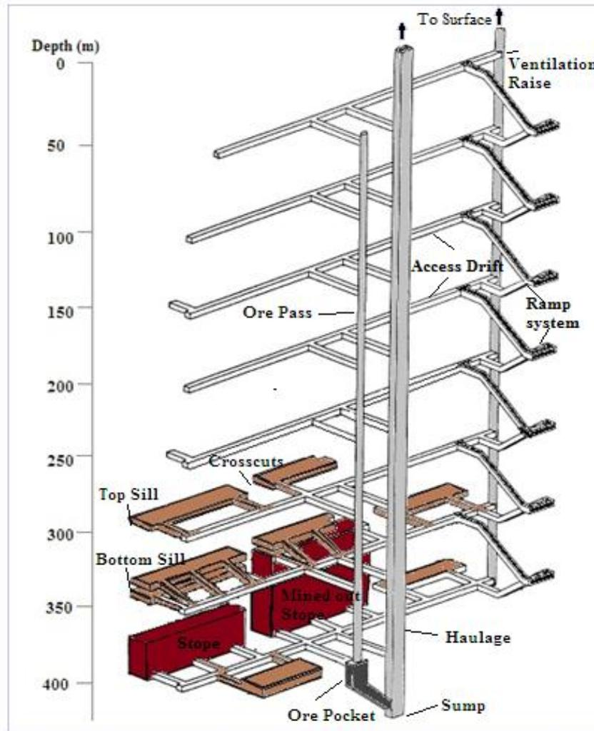
Fig 9: Schematic design of Underground mine for Khalashpir coal field (Coal seam I )
