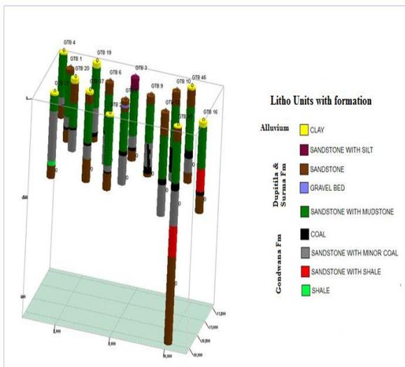
**Fig 2: 3D multi-log system showing the major litho units distribution**
