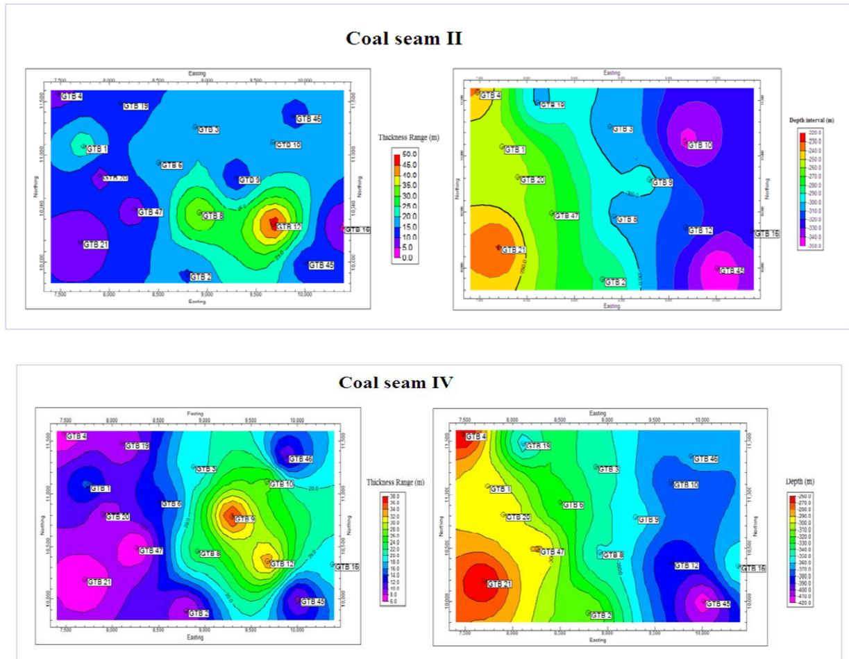
**Fig 5: Showing the thickness and depth variation of coal seam I, II and IV throughout the basin (using software Rockware15)**
