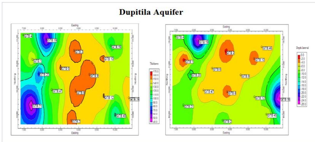
**Fig 6: Upper Dupitila aquifer thickness and Depth variation (using software Rockware15)**
