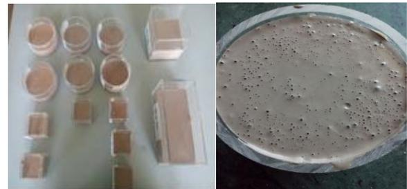
**Figure 2 Metakaolin Geopolymer Foamed Slurry**
