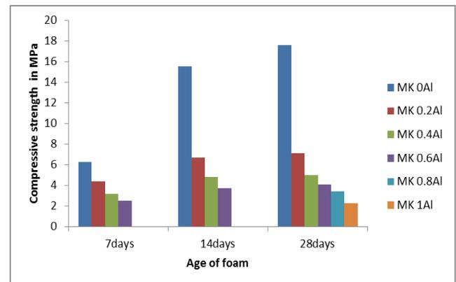
**Figure.3 Compressive Strength of Metakaolin Geopolymer Foam**
