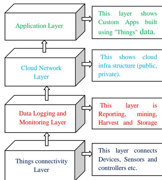
**Fig 1 : Four Layer Structure of IIoT**
