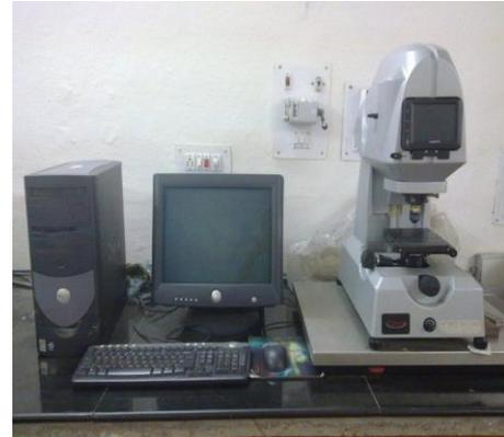
**Fig 1.8: Optical profile meter**
