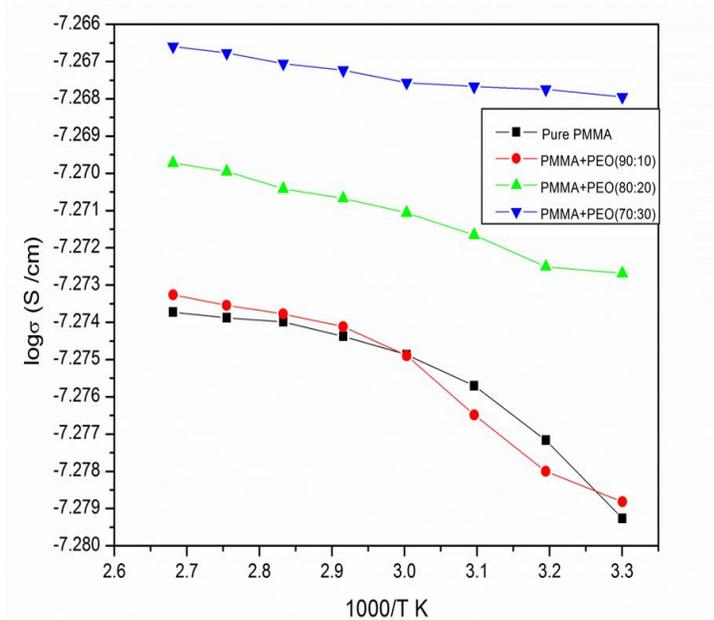
**Figure 3. DC conductivity of Pure PMMA and different concentrations of PMMA and PEO**
