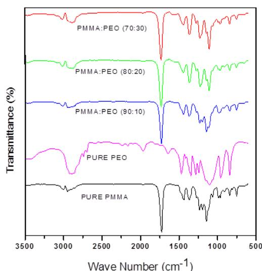
**Figure 1. FTIR analysis of Pure PMMA, PEO and their ratios**
