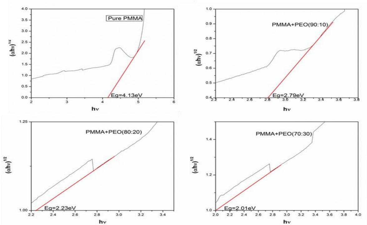
**Figure 2. UV plots of Pure PMMA and different concentrations of PMMA and PEO**
