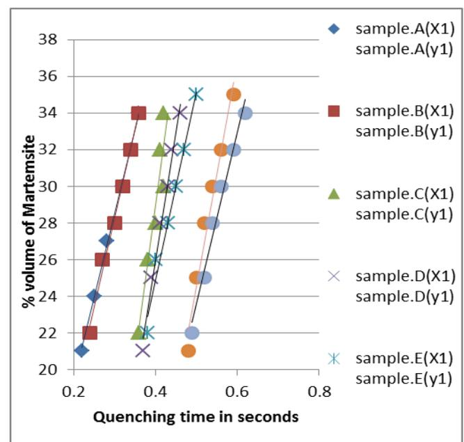
Figure-8, Relationship between quenching time and % volume of marten-site
