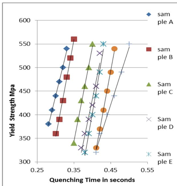
Figure-7, Relationship between yield strength and quenching time
