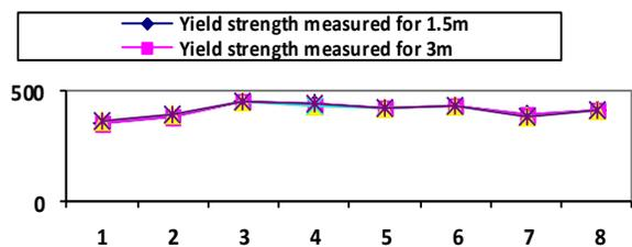
**Figure-3 Re-bars yield strength variations at different length in Self-Tempering sequence**
