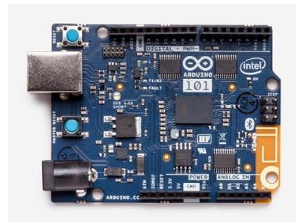
**Figure 3 Arduino 101 microcontroller board**
