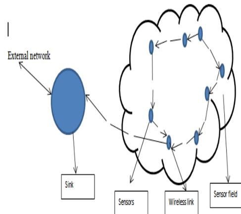
**Figure 1.1 Basic Structure of WSN**
