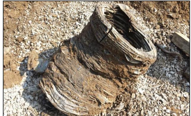
Figure 2. Compressed CMP
