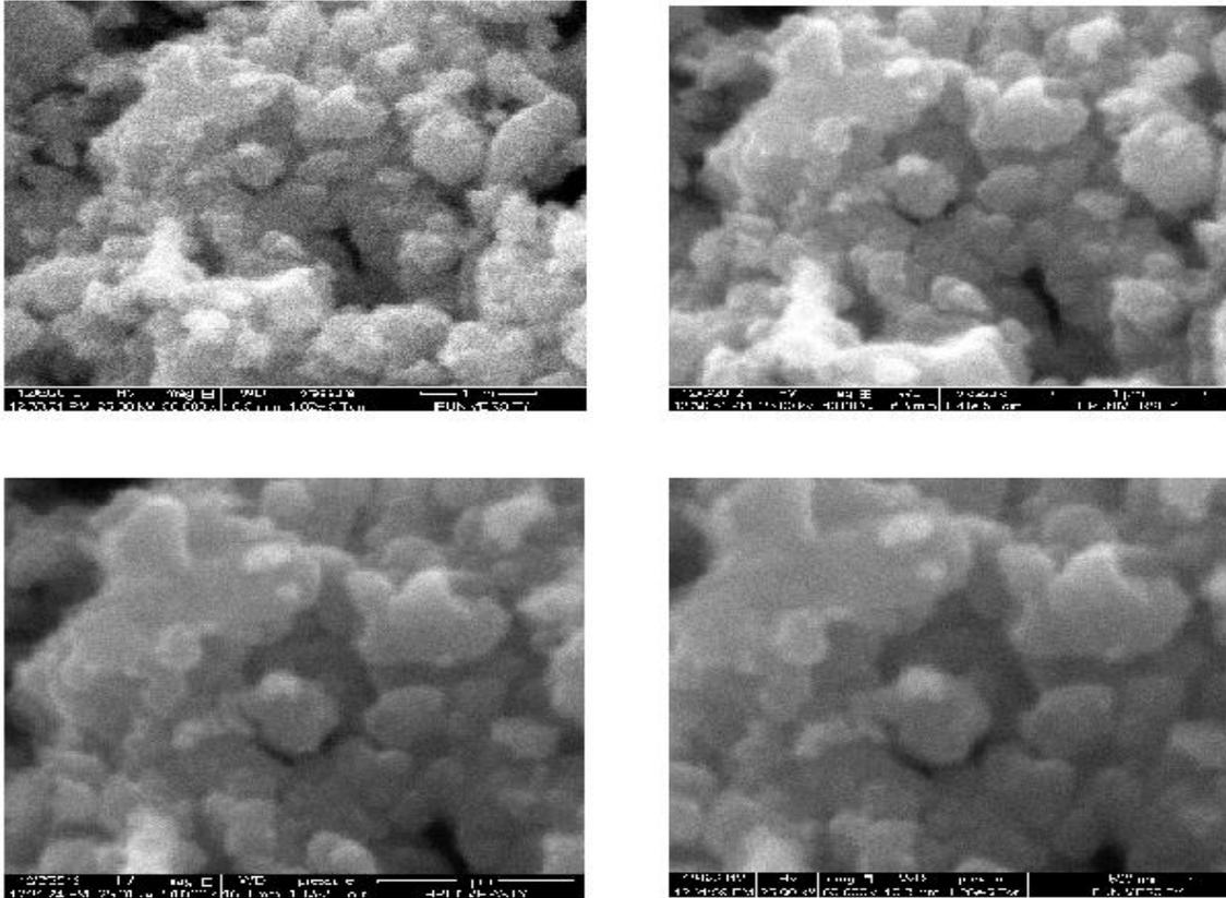
Fig.(2) SEM morphology images for nano-crystalline Co doped SnO<sub>2</sub> powders annealed at (a) 350°C, (b)450°C, (c) 550°C, (d) 650°C
