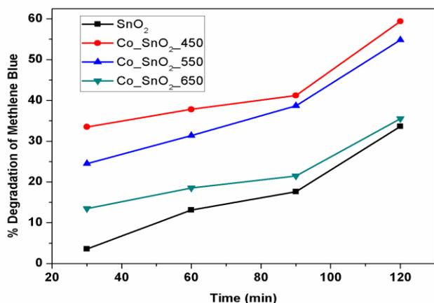
Fig.(4) Degradation % of Methylene Blue for pristine & Co doped SnO<sub>2</sub> annealed between 450°C to 650°C
