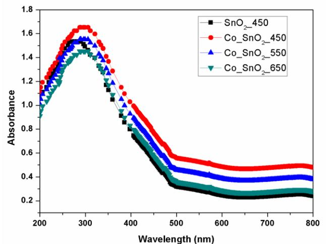
Fig.(3) Absorption Spectra of pristine & Co doped SnO<sub>2</sub> annealed between 450°C to 650°C
