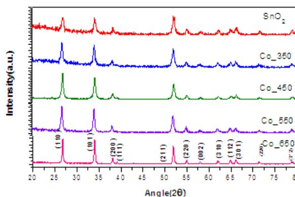
Fig.(1) XRD patterns of Co doped SnO<sub>2</sub> (x=0.005) annealed between 350<sup>0</sup>C to 650<sup>0</sup>C
