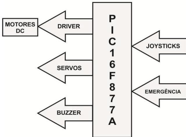
Figure VIII- Control system diagram
