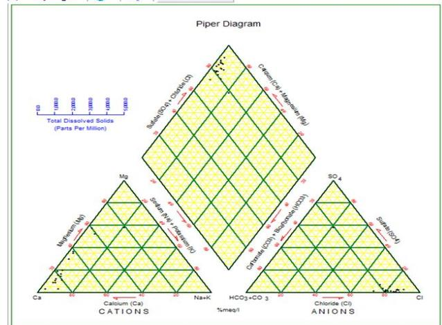
**Fig 5: Piper trilinear diagram for major ion chemistry for Post-monsoon (2015) of the study area.**
