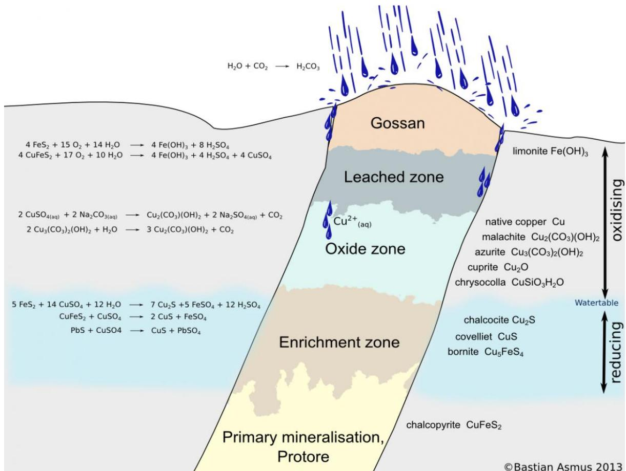
Figure 3: Schematic diagram of deposits formed due to oxidation and secondary enrichment (after Asmus, 2013).
