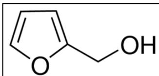
Fig. 1 Structure of Furfural Alcohol
