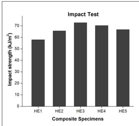
Figure 5: Impact strength of HE composites
