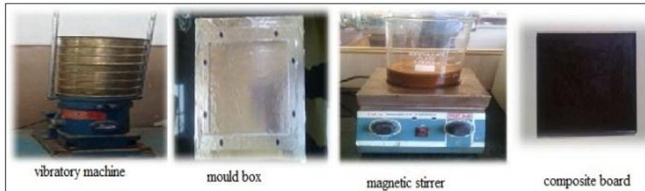
**Figure 2: Process for fabrication of composite boards**
