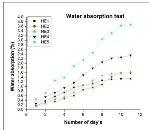
Figure 8: Water absorption of HE composites
