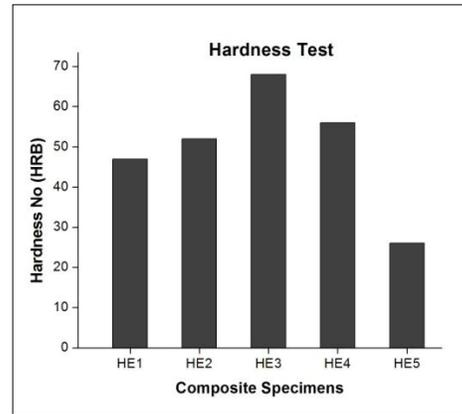
Figure 6: Hardness of HE composites
