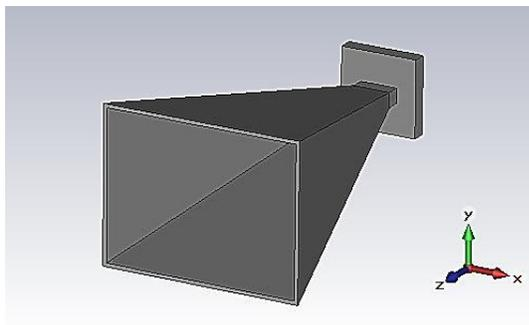
**Figure 6: Pyramidal Horn Antenna Designed in CST MW**
