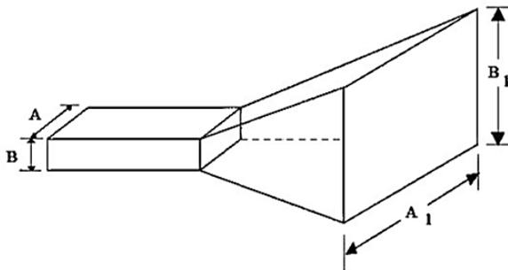
Figure 2: Pyramidal Horn Antenna
