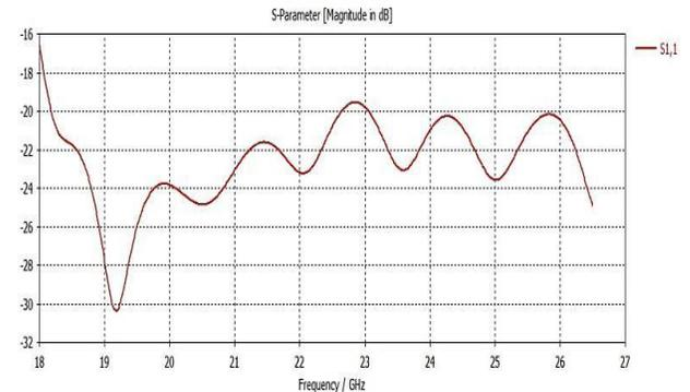
**Figure 7: Return loss vs. Frequency.**
