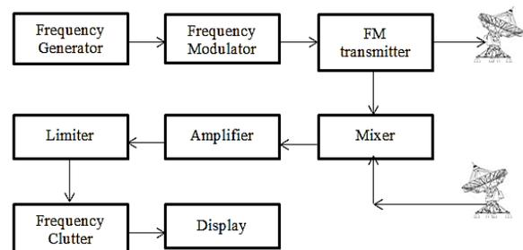
**Figure 1: Block diagram of FMCW Radar**
