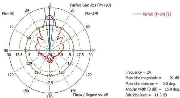
**Figure 9: 2D Plot of Radiation Pattern (dB)**
