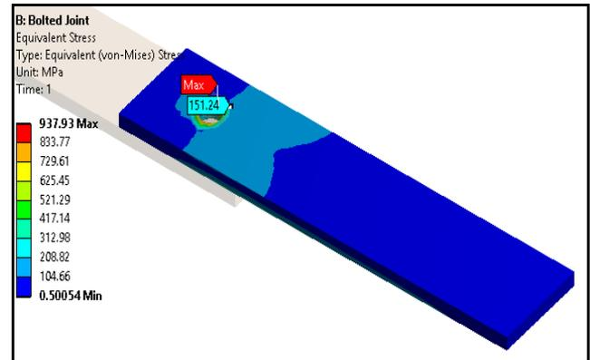
**Fig.11. Von Mises stress plot at maximum load**
