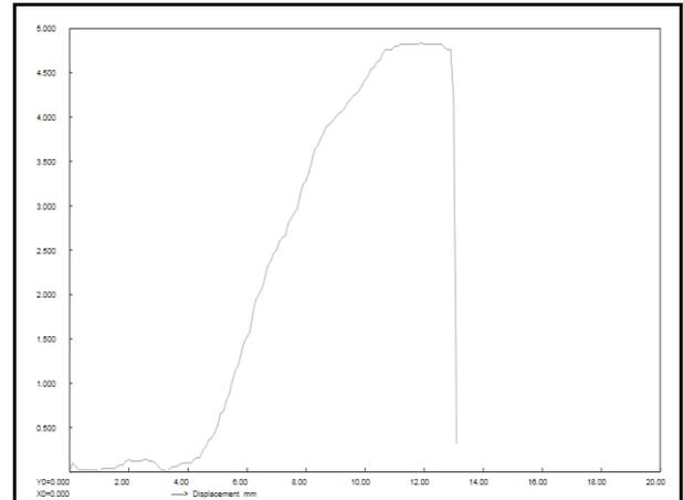
**Fig.23. Graph of load vs displacement at bolted joint**
