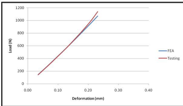
**Fig.25. Comparative Graph of Load vs deflection for bonded joint**
