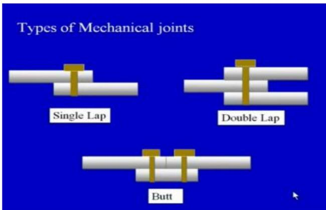
**Fig.4 Type of Mechanical joints[11]**
