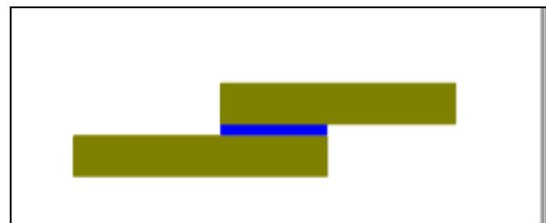
Fig 1. Adhesive joint (Permanent Joint) [11]
