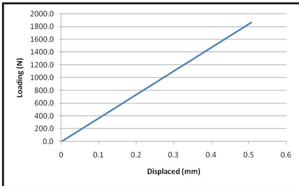
**Fig.10. FEA graph of Riveted joint Load vs deflection**
