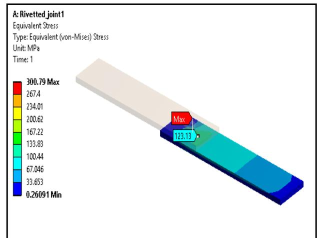
**Fig.8. Von Mises stress plot at specimen**
