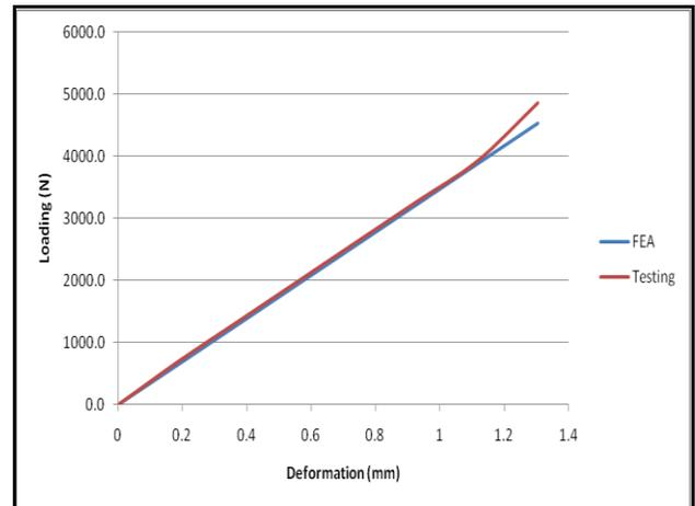
**Fig.27. Comparative Graph of Load vs deflection for bolted joint**
