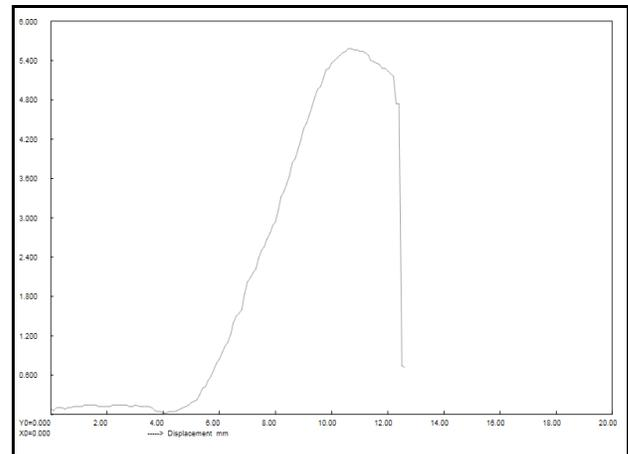
**Fig.24. Graph of load vs displacement for hybrid joint**
