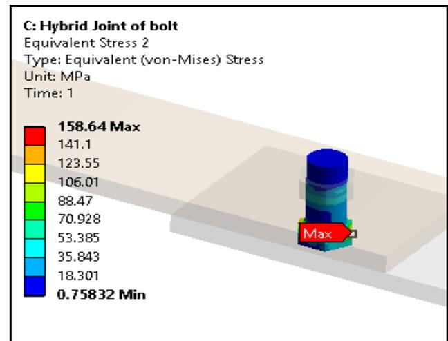
**Fig.16. Stress plot at the bolt**
