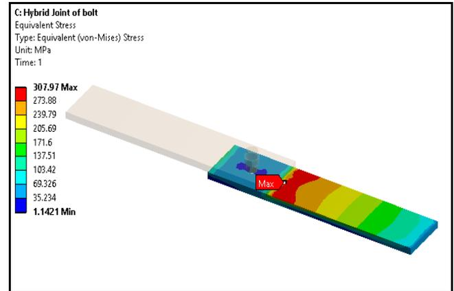
**Fig.15. Von mises stress plot at GFRP plate**
