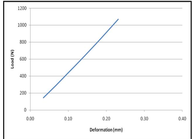
**Fig.7. FEA graph of bonded joint Load vs deflection**
