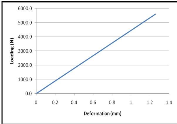
**Fig.18. FEA graph of Hybrid joint Load vs deflection.**
