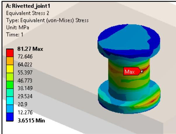
**Fig.9. Von Mises stress plot at Rivet**
