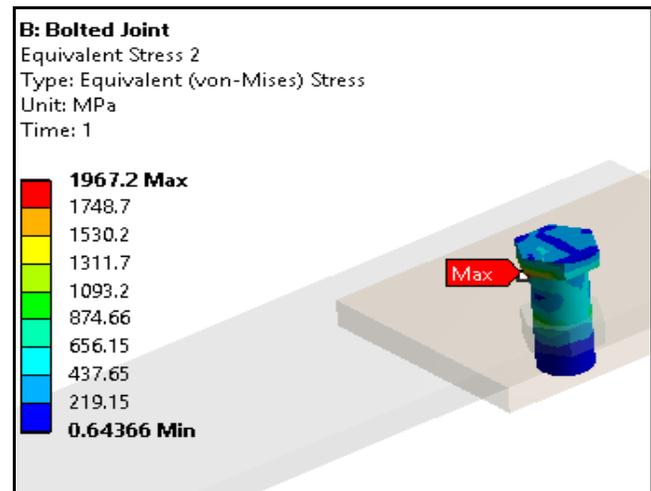
**Fig.12. Von mises stress plot at bolt**
