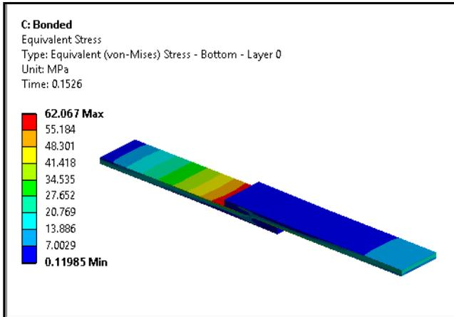
**Fig.5. Von Mises stress plot at peak load bonded joint**
