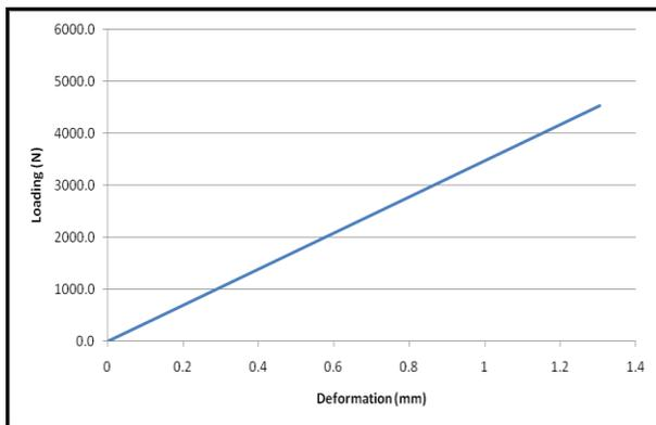
**Fig.14. FEA graph of Bolted joint Load vs deflection**
