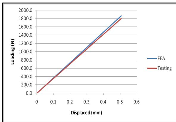
**Fig.26. Comparative Graph of Load vs deflection for Riveted Joints**
