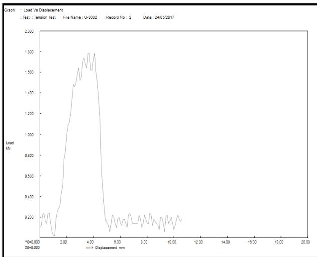
**Fig.22. UTM testing results for Riveted Joints**
