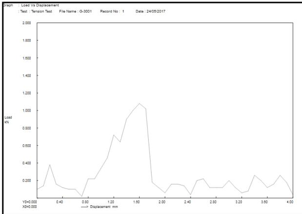
**Fig.21. Testing graph of bonded material test Load vs deflection**
