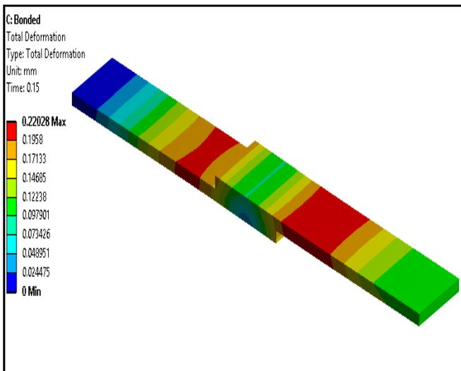
**Fig.6. Deformation at maximum load**
