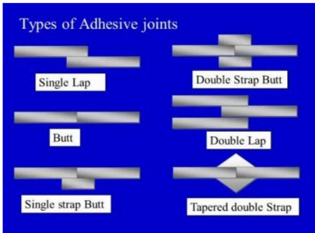
**Fig.3 Type of adhesive joints [11]**
