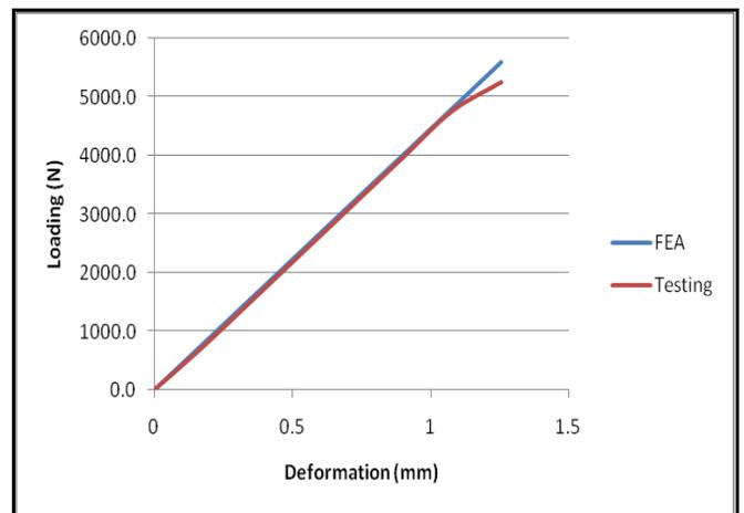
**Fig.28. Comparative Graph of Load vs deflection for hybrid joint**
