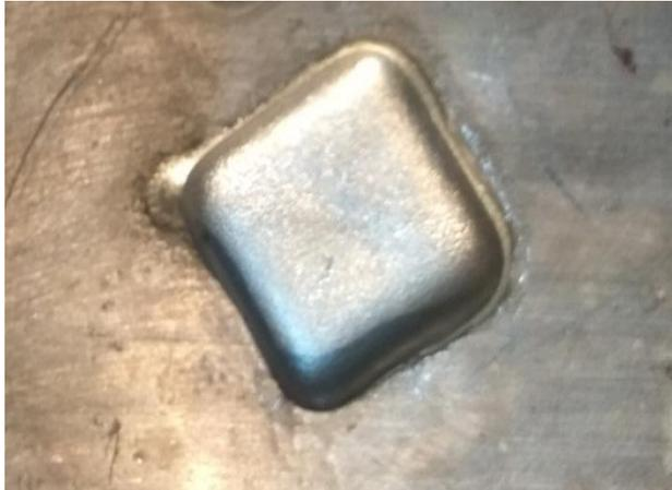
**Figure-8 Profile of work piece with insulated tool.**
