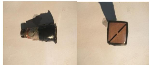
**Figure-7 Insulated tool as used in ECM experiments**
