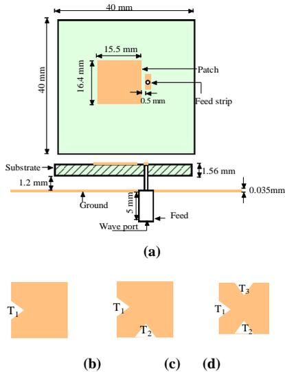
**Fig.1 (a) Antenna1 without any triangular cut (b) Antenna2 with one triangular cut  $T_1$  (c) Antenna3 with two triangular cuts  $T_1$  and  $T_2$  (d) Antenna4 with three triangular cuts  $T_1$ ,  $T_2$  and  $T_3$**
