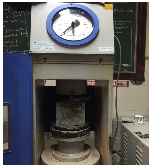
Fig 1 Testing for Compressive strength
