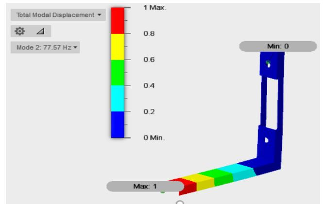
**Fig.20. Mode shape plot iteration 2 model mode 2**
