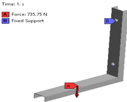
**Fig.23. Loading of 735.75 N on the side and fixed support at holes**
