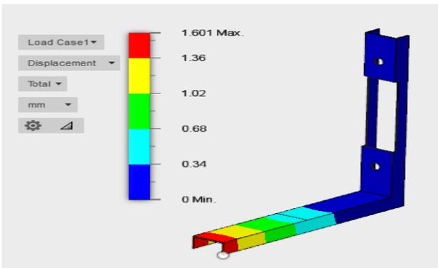
**Fig.18. Total deformation plot Iteration 2**
