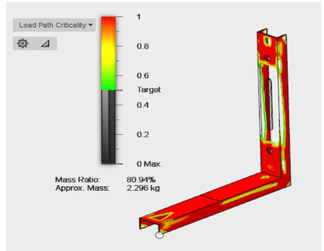
**Fig.14. Load Criticality path for Iteration 1**
