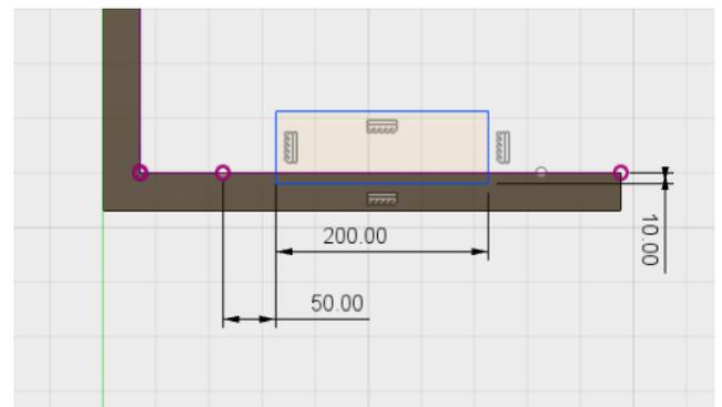
**Fig.16. Sketch for modification of L bracket Iteration 2 design**
