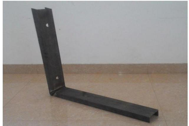
**Fig.30. Basic model of the fuel tank mounting bracket**
