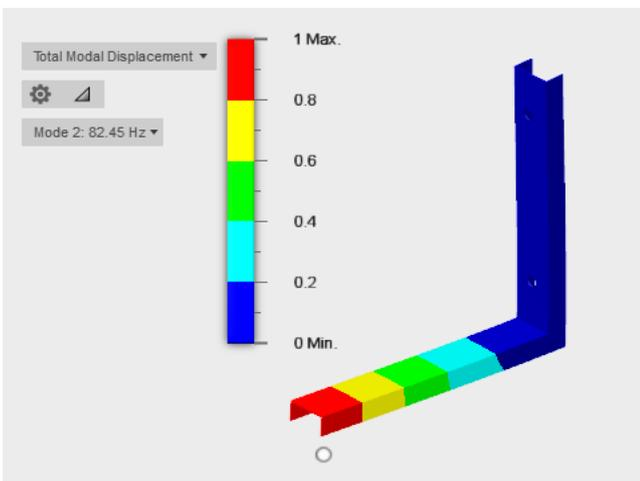
**Fig.5. Mode shape plot at second natural frequency 82.45 Hz.**
