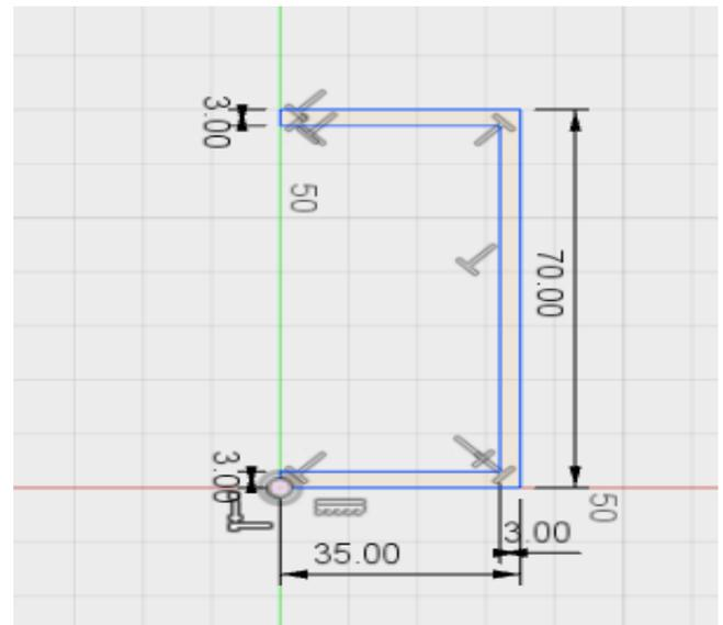
**Fig .2. Cross section of the bars used for modeling**
