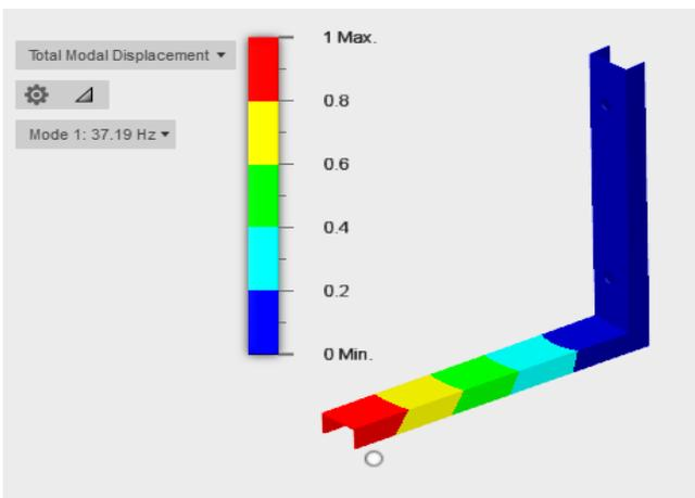
**Fig.4. Mode shape plot at first frequency 37.2 Hz**
