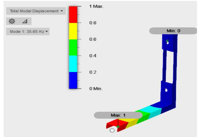
**Fig.19. Mode shape plot iteration 2 model mode 1**
