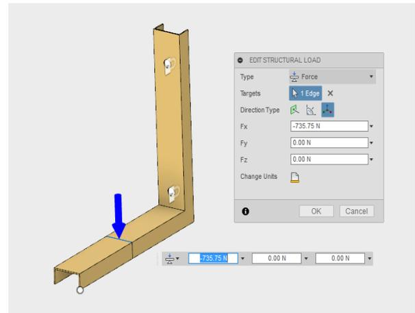
**Fig.6. Loading condition and boundary condition of the bracket.**
