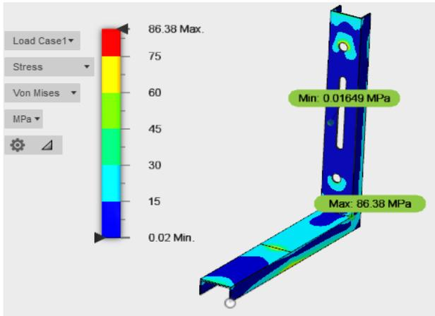
**Fig.12. Iteration 1 Stress plot (Mpa).**
