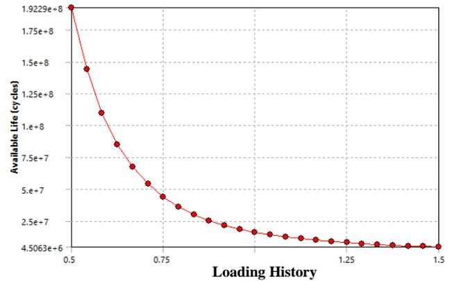
**Fig.26. Fatigue sensitivity graph for baseline**
