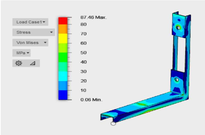
**Fig.17. Von Mises stress plot Iteration 2**
