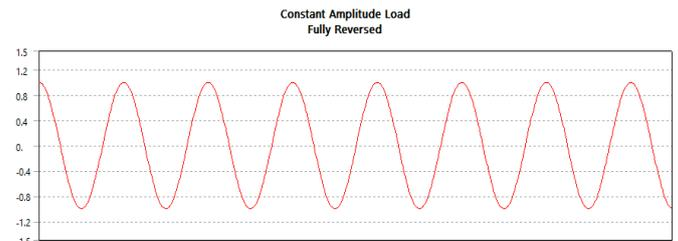
**Fig.21. Loading for fatigue analysis**
