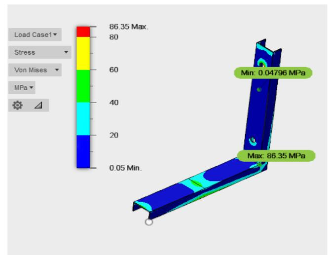
**Fig.7. von Mises stress plot at static analysis.**
