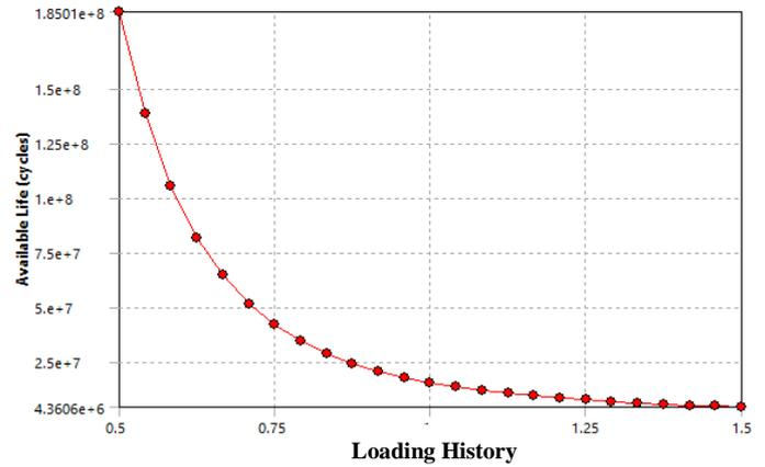
**Fig.29. Fatigue sensitivity plot iteration 3**
