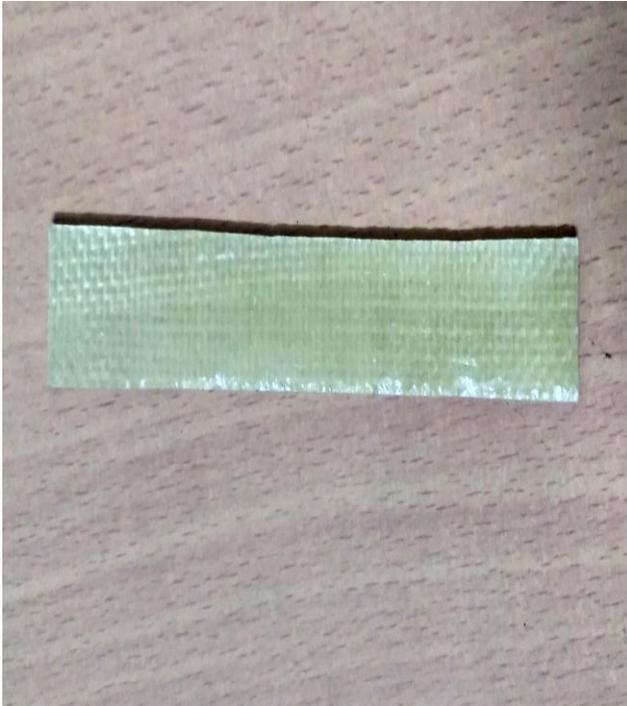
**Fig.1. Composite Beam Specimen (150x20x3)**
